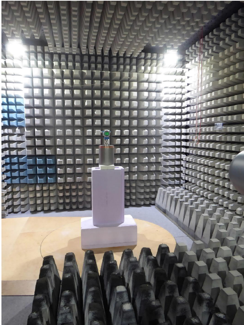
Test setup fully anechoic chamber (1 GHz to 12 GHz)
