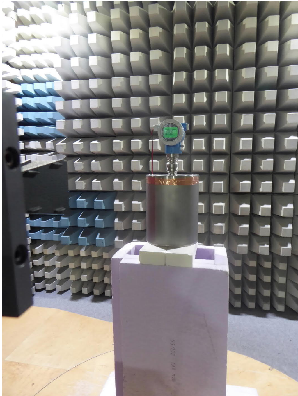
Test setup fully anechoic chamber with (>26.5 GHz)
