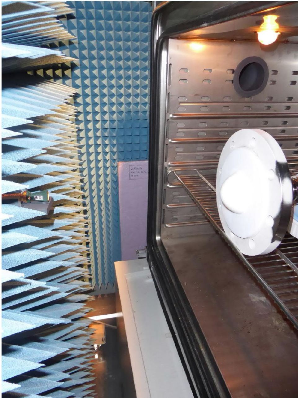
Test temperature chamber with EUT 5 (isolation removed)
