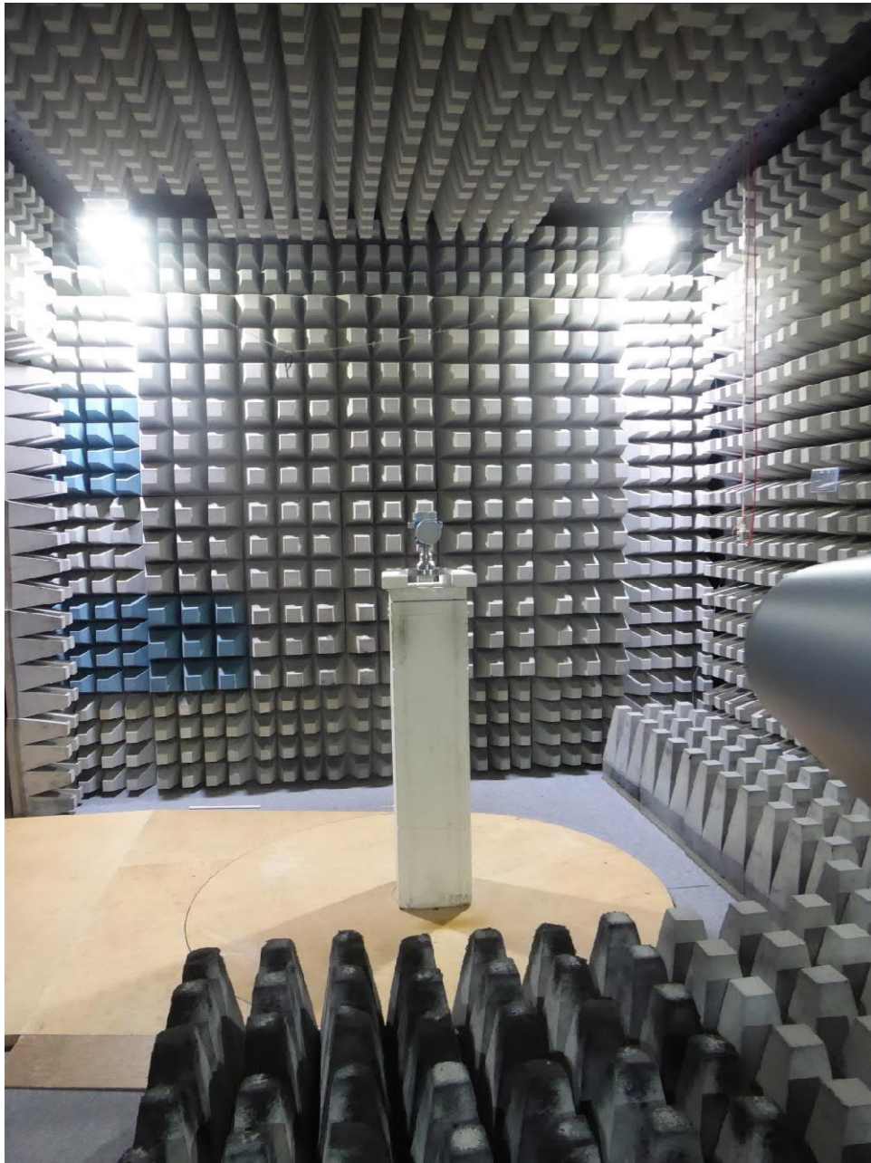
Test setup fully anechoic chamber with EUT 5 (<40 GHz, position 1)
