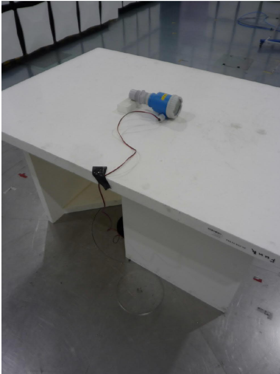
Test setup semi anechoic chamber with EUT 1 (position 1)
