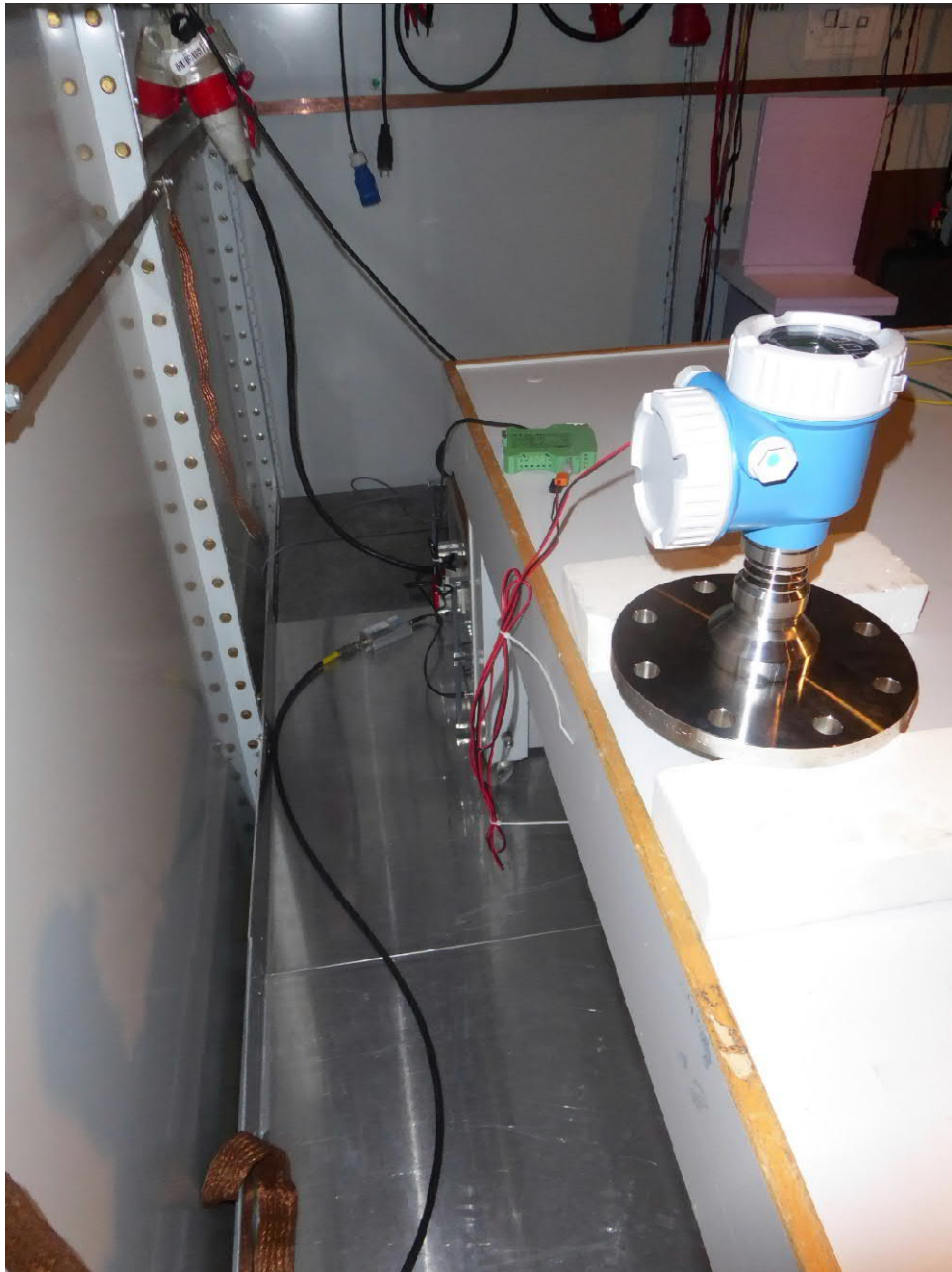
Test AC power line conducted emissions with EUT 5
