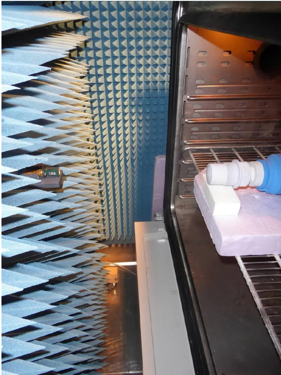
Test temperature chamber with EUT 1 (isolation removed)
