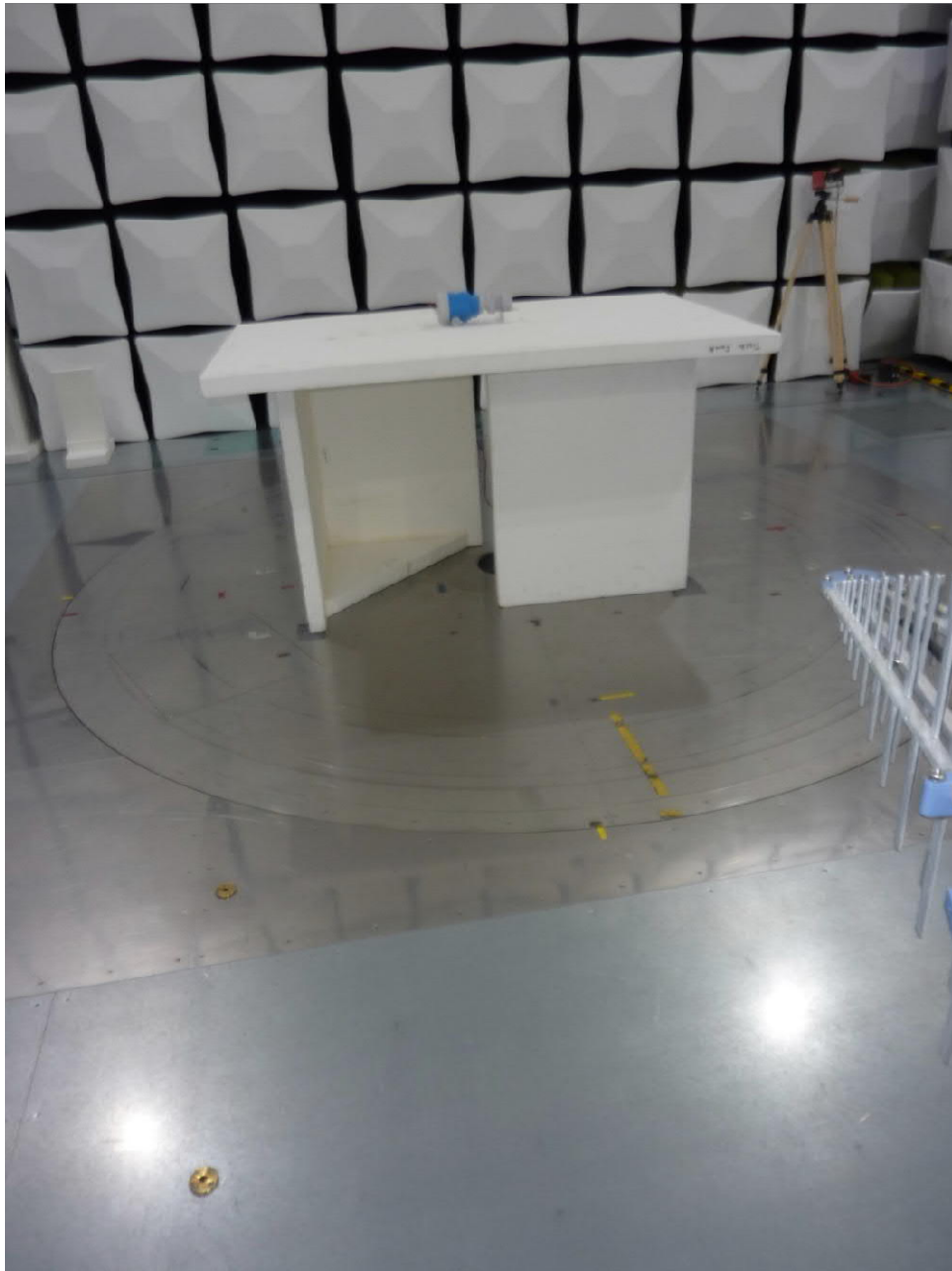
Test setup semi anechoic chamber with EUT 1 (<1 GHz, position 1)
