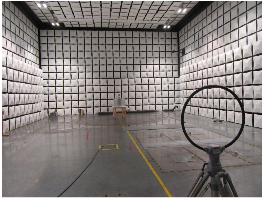
Figure 4 - Test setup for radiated emission on TLPR
