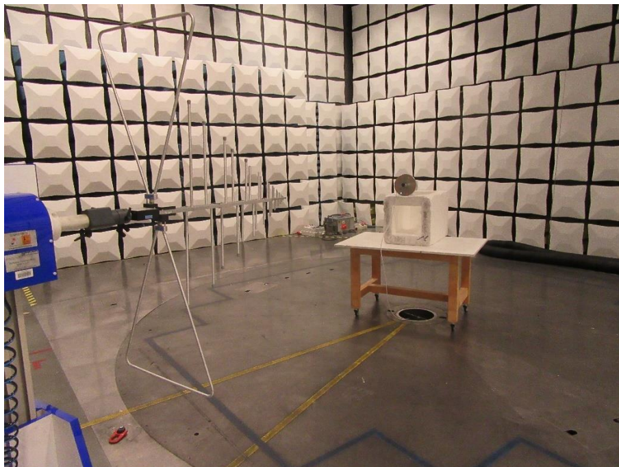
Figure 9 - Test setup for radiated emission on LPR
