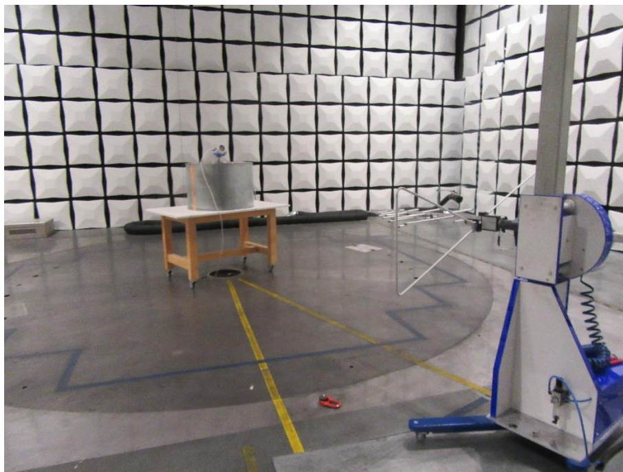
Figure 5 - Test setup for radiated emission on TLPR
