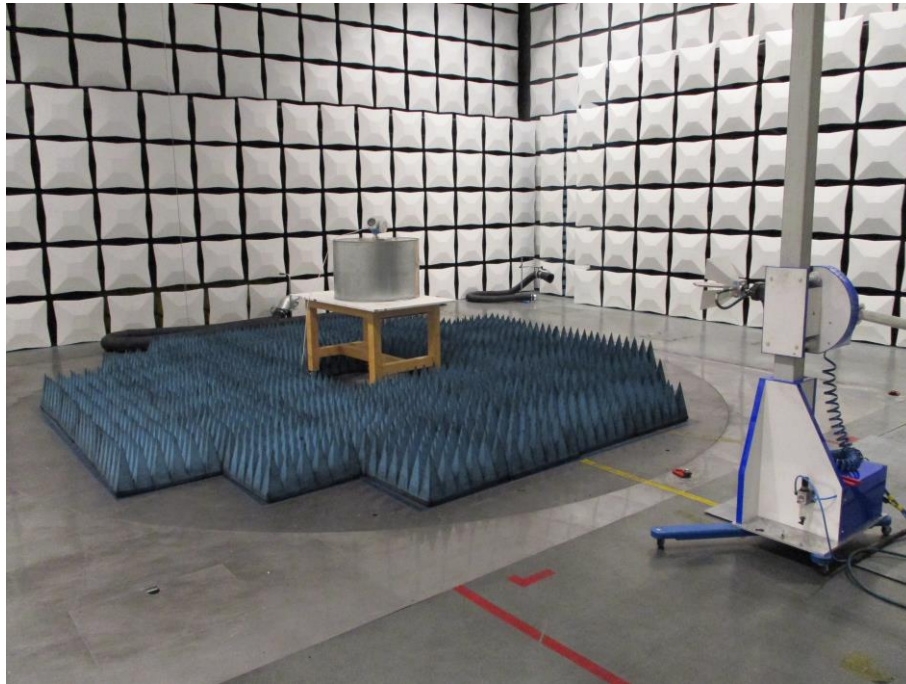
Figure 6 - Test setup for radiated emission on TLPR
