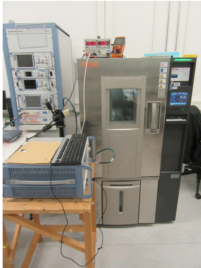
Figure 1 - Test setup for testing under extreme conditions (frequency stability)
