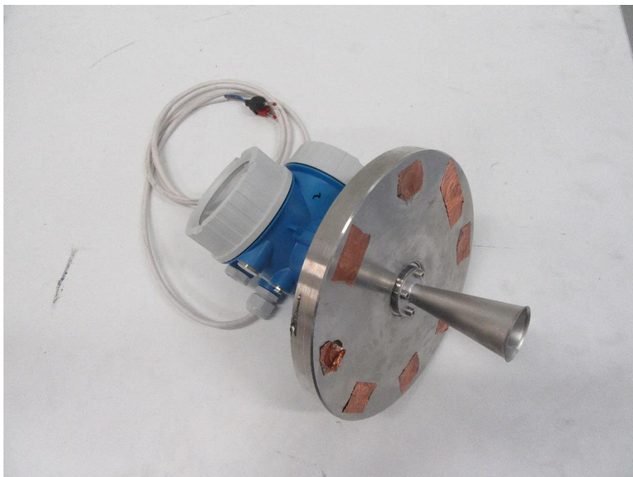
Figure 1 – EUT P2 (FMR50 with antenna Horn 100mm/4" PP clad)
