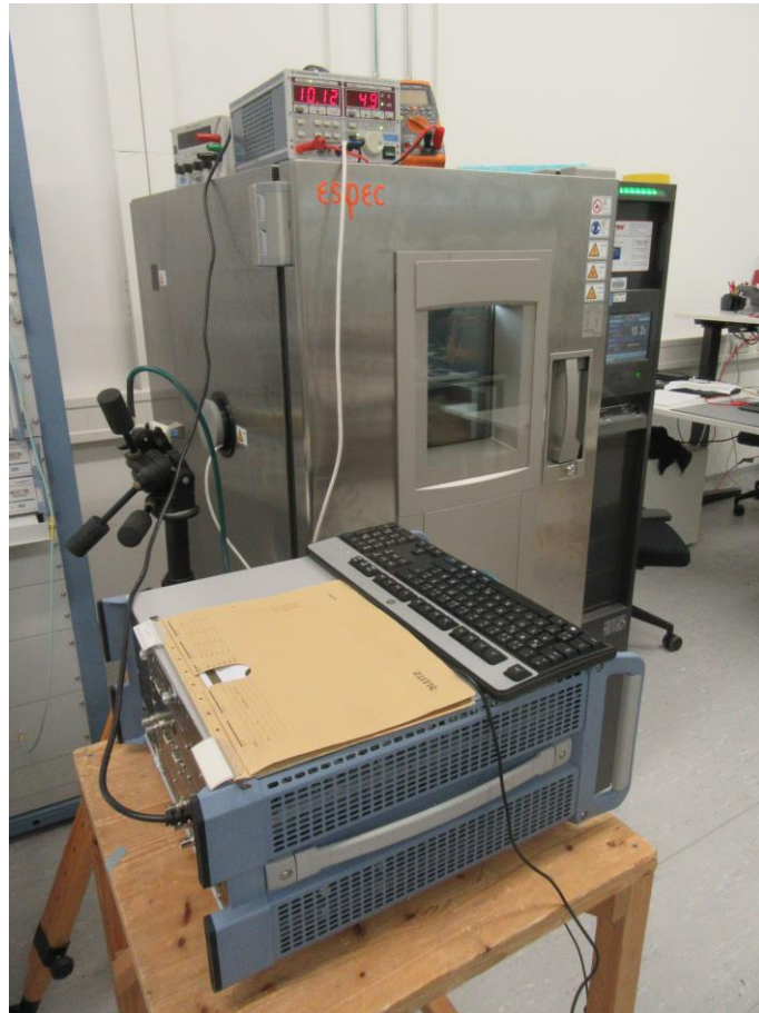
Figure 14 - Test setup for testing under extreme conditions (frequency stability)
