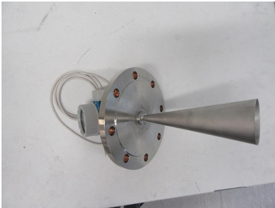
Figure 3 – EUT P5 (FMR52 with antenna Horn 80mm/3" flush mount)
