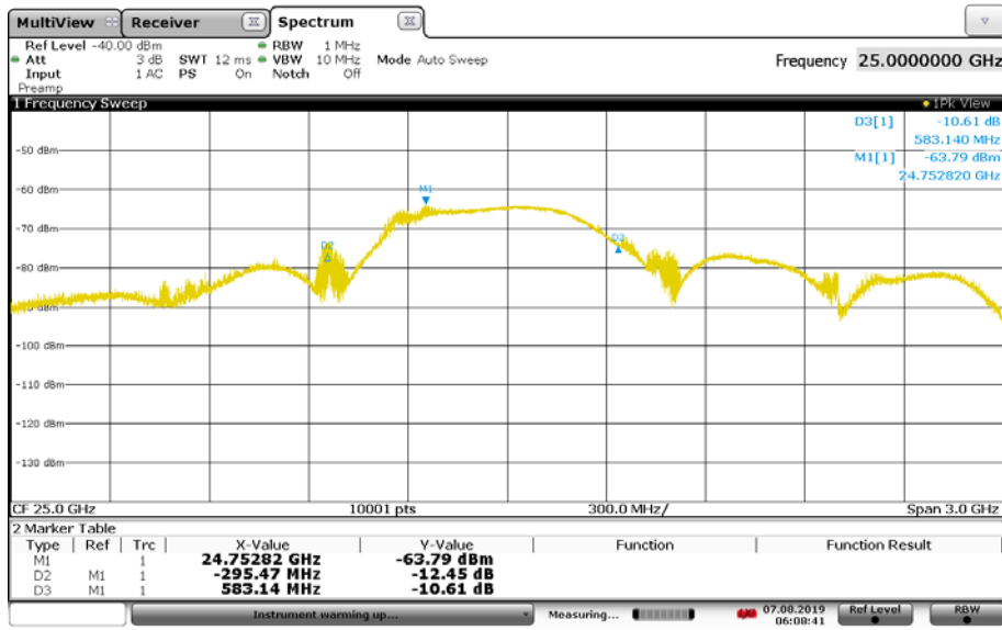
Fundamental Emission -10 dB Bandwidth – 24.0V DC / +20°C
