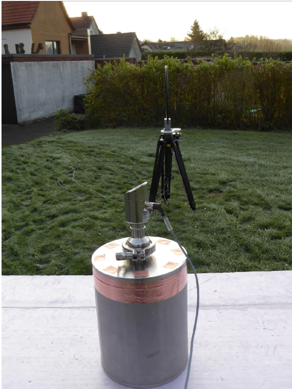
Test setup semi anechoic chamber with EUT 4 (9 kHz to 30 MHz, final)
