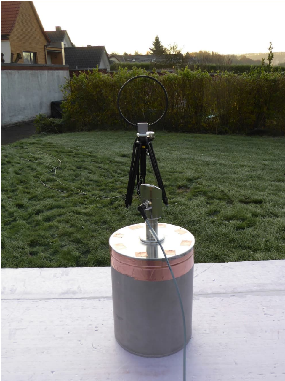
Test setup semi anechoic chamber with EUT 1 (9 kHz to 30 MHz, final)
