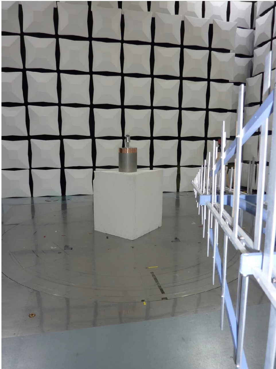
Test setup semi anechoic chamber with EUT 1 (30 MHz to 1 GHz)
