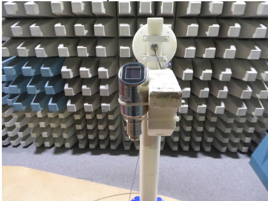
EUT on positioner Test setup fully anechoic chamber M20 Preliminary and final measurement
