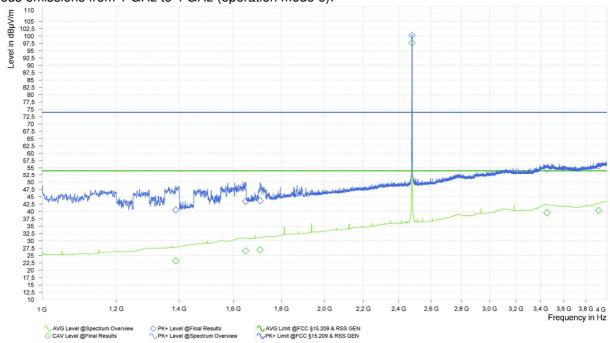
Spurious emissions from 1 GHz to 4 GHz (operation mode 6):
