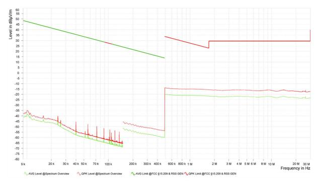
Spurious emissions from 9 kHz to 30 MHz (operation mode 5 – Position 2):
