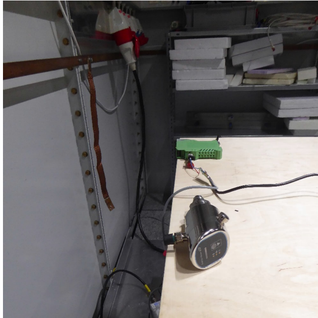
Test setup shielded room M4 Preliminary and final measurement 150 kHz – 30 MHz
