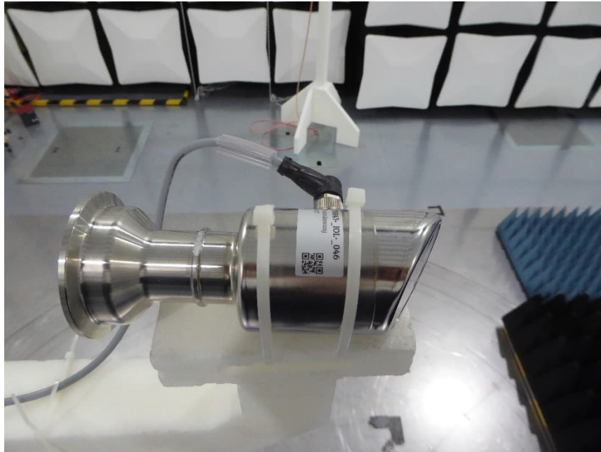
EUT on positioner Test setup semi-anechoic chamber with ground absorbers M276 Preliminary and final measurement 1 GHz – 18 GHz
