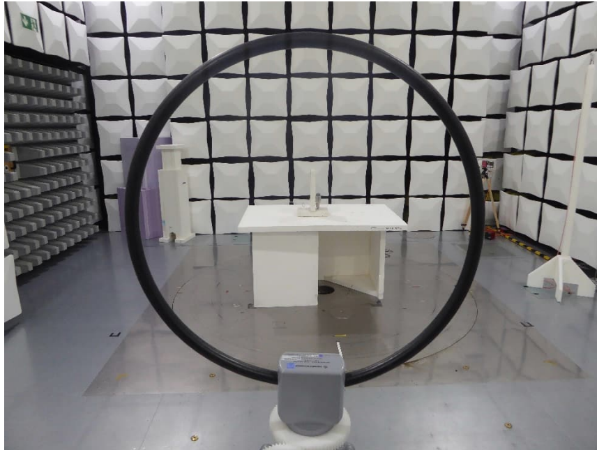
Test setup semi-anechoic chamber M276 Preliminary measurement
