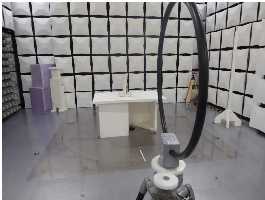
Antenna Position 2 – perpendicular Test setup semi-anechoic chamber M276 Preliminary measurement
