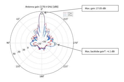
(\*) Backlobe gain means antenna gain in the half-sphere opposing the intended installation direction of the radar device.
