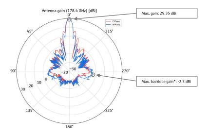
(\*) Backlobe gain means antenna gain in the half-sphere opposing the intended installation direction of the radar device.
