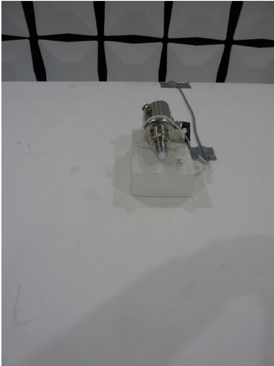
Test setup semi anechoic chamber with EUT 6b (9 kHz to 1 GHz), position 2
