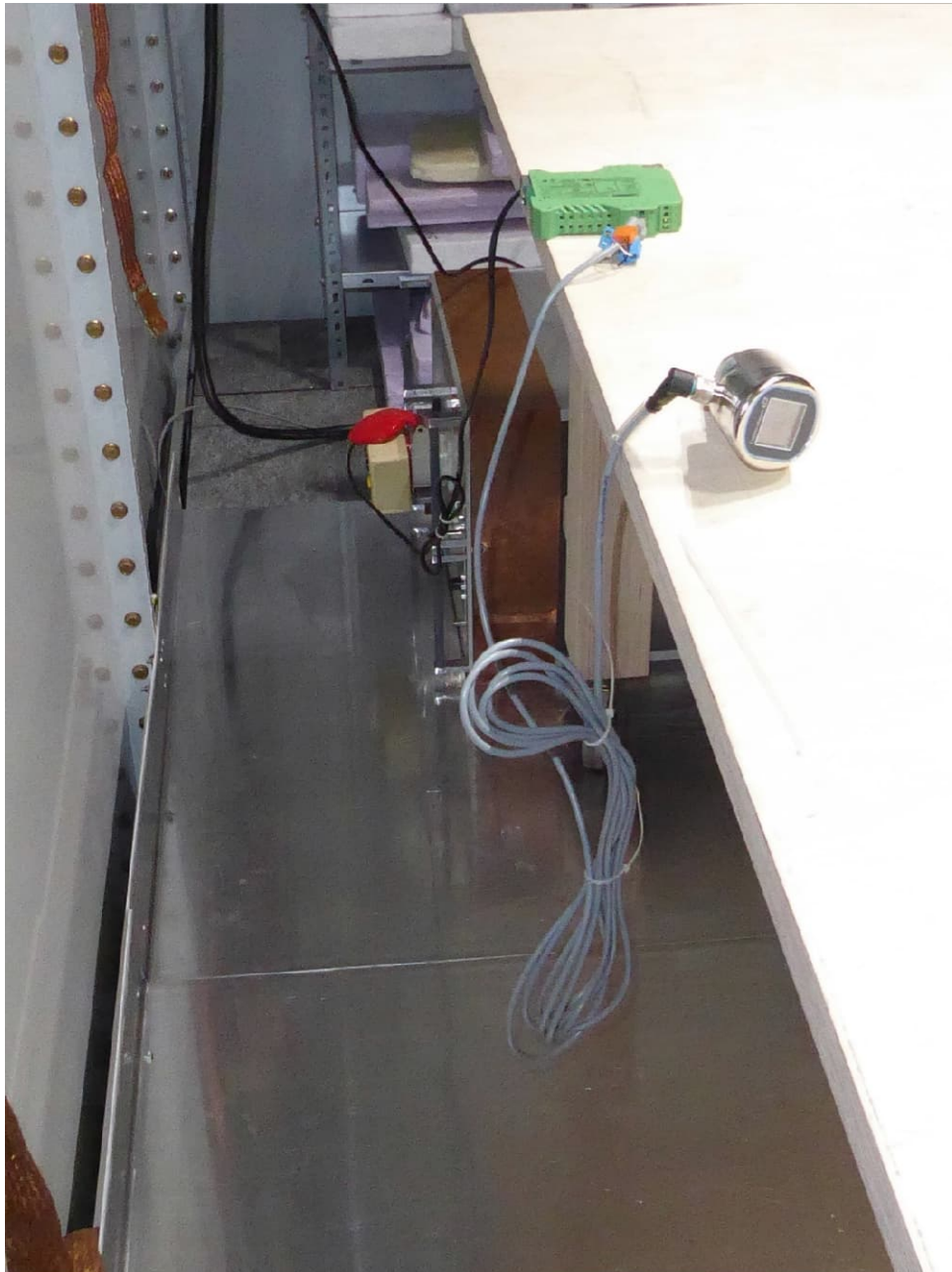
Test setup shielded chamber with EUT 5b (conducted emissions on power supply line)
