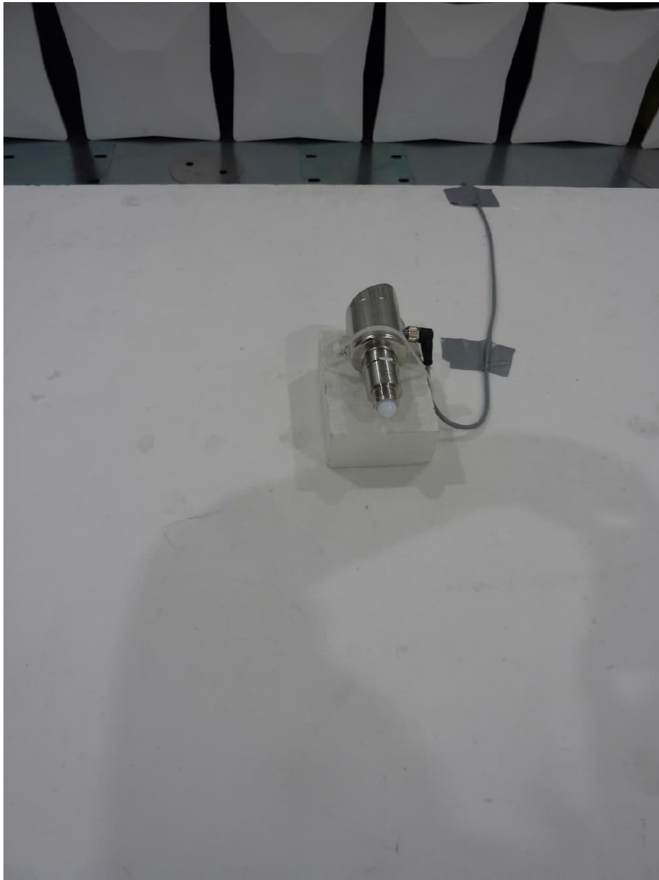
Test setup semi anechoic chamber with EUT 5b (9 kHz to 1 GHz), position 2
