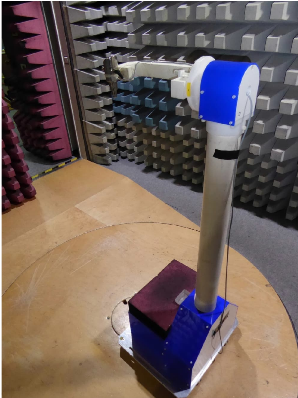
Test setup fully anechoic chamber with EUT 6b (<40 GHz)
