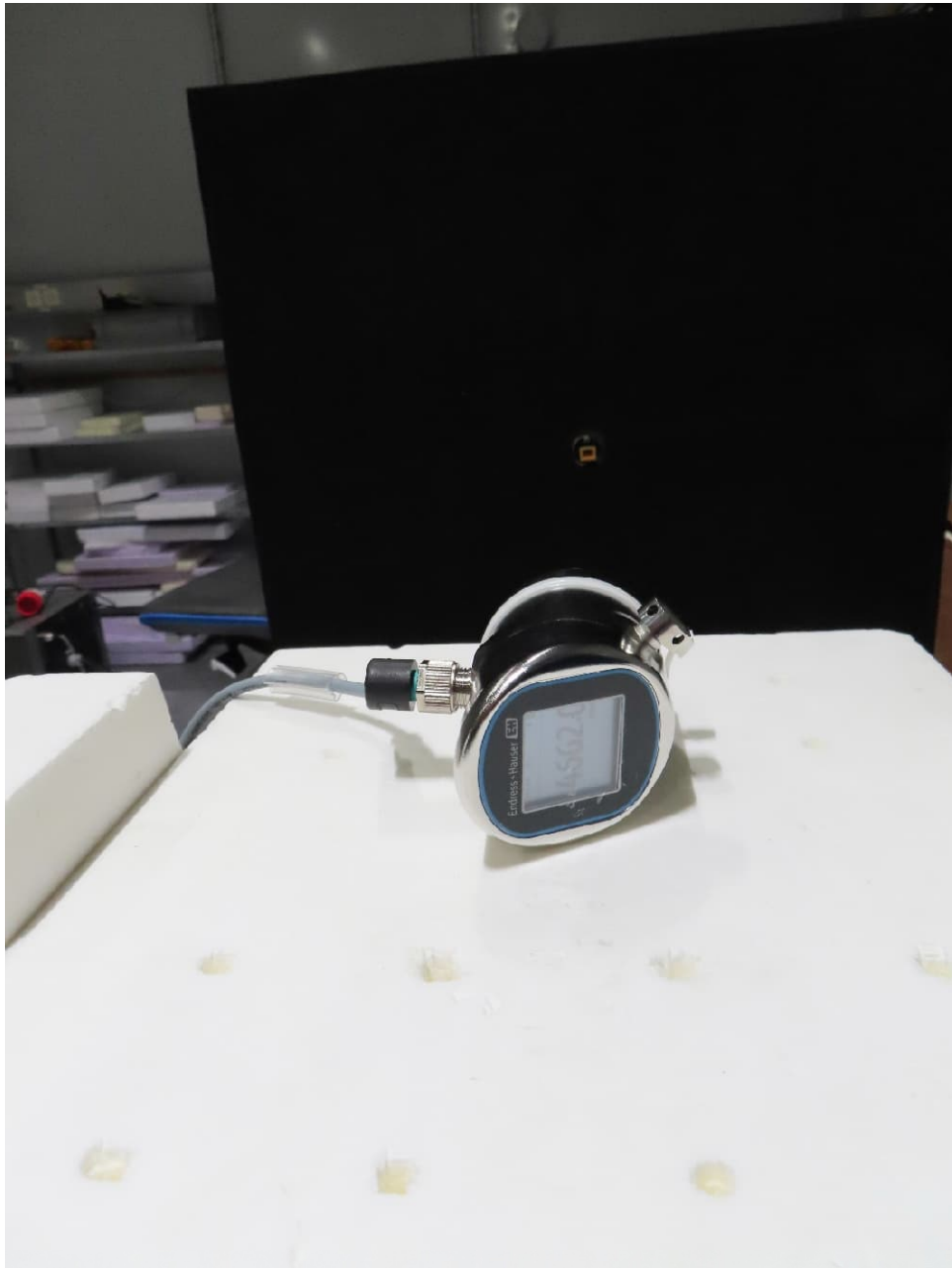
Test setup fully shielded chamber with EUT 6b (>330 GHz)
