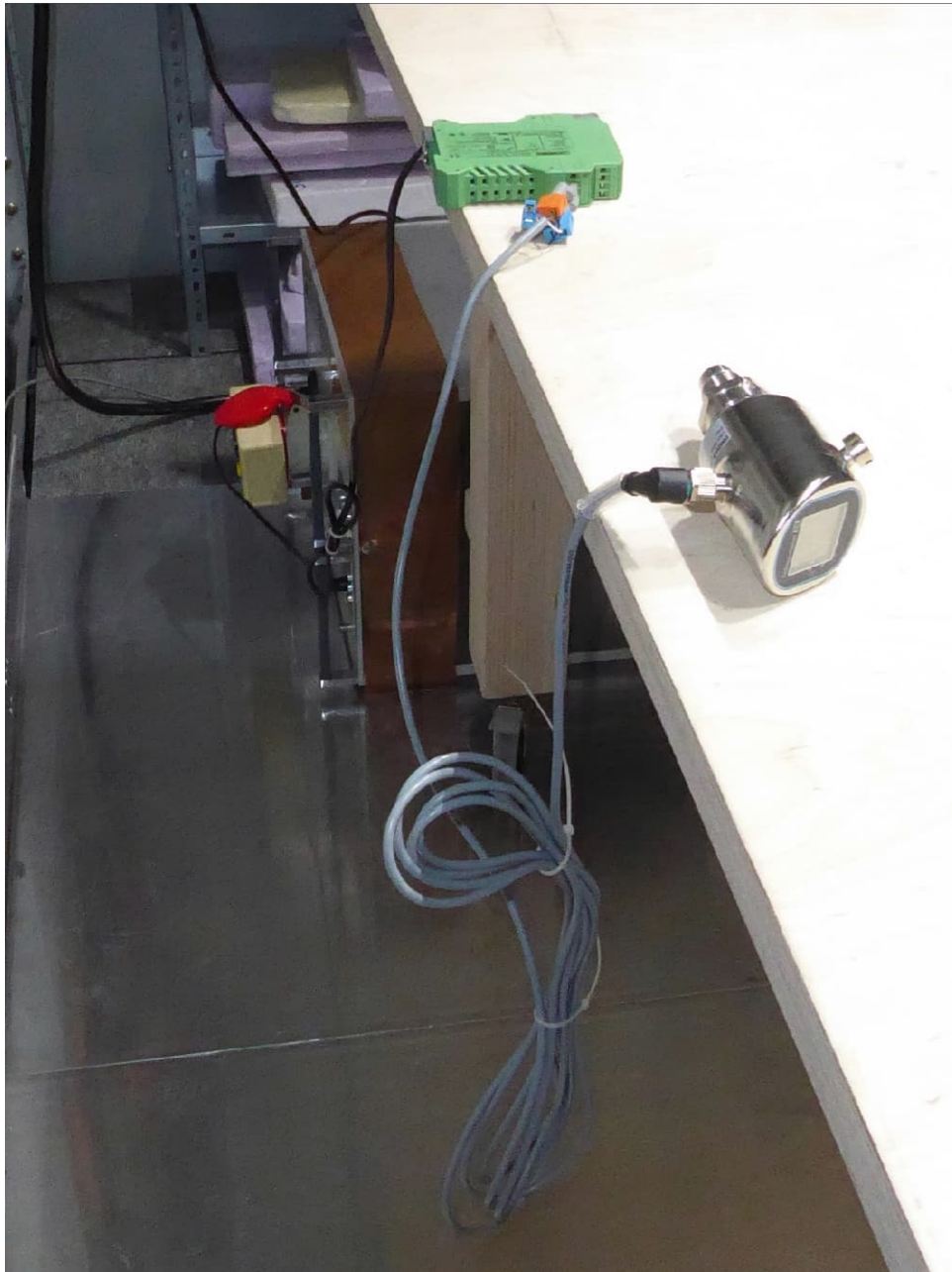
Test setup shielded chamber with EUT 6b (conducted emissions on power supply line)
