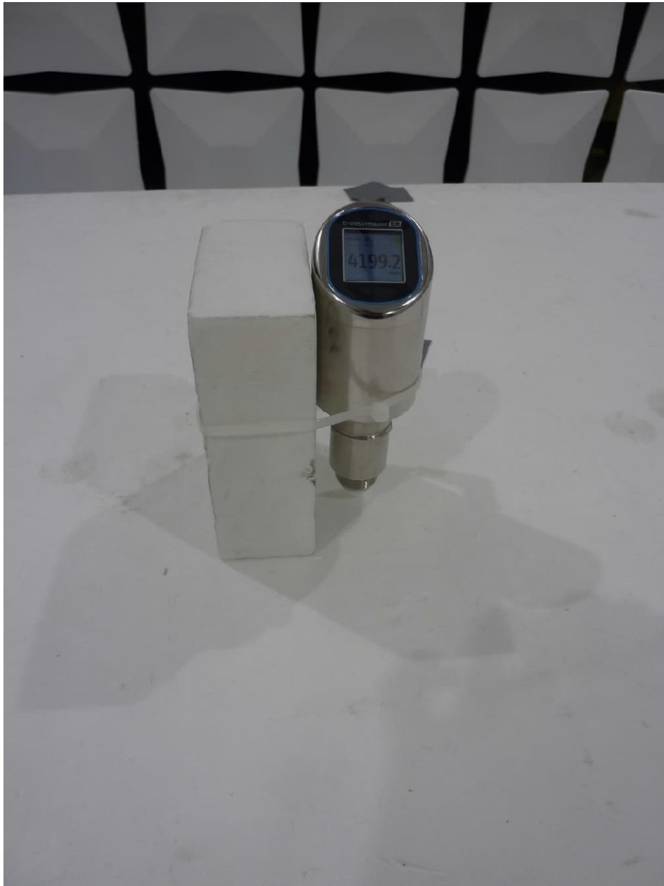
Test setup semi anechoic chamber with EUT 5b (9 kHz to 1 GHz), position 1
