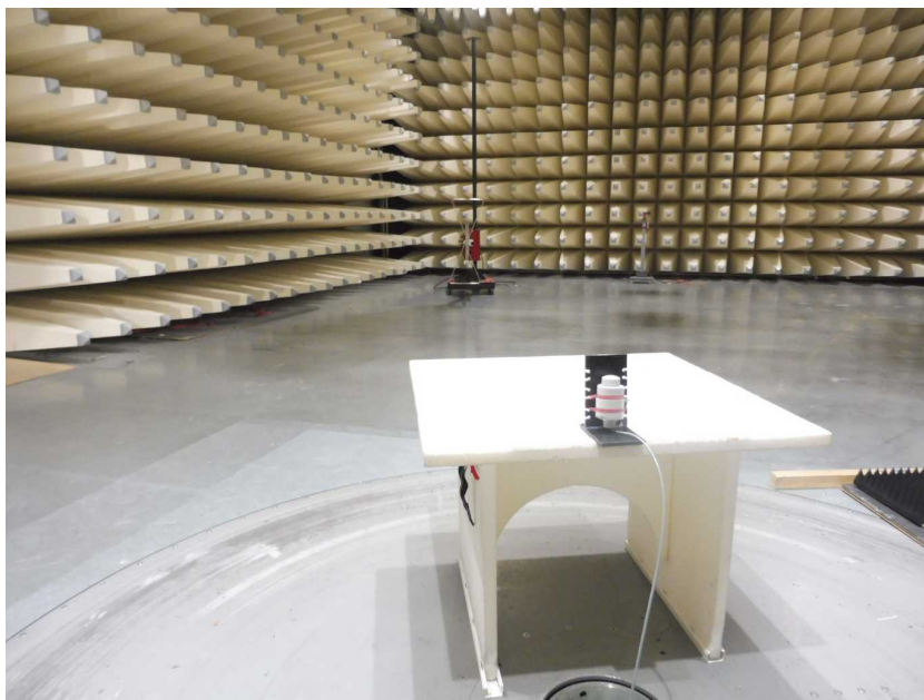
Photo 8: EUT at the semi-anechoic chamber
