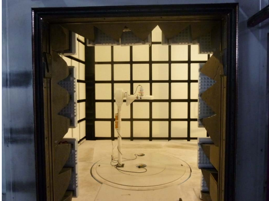
Photo 1: EUT at the anechoic chamber
