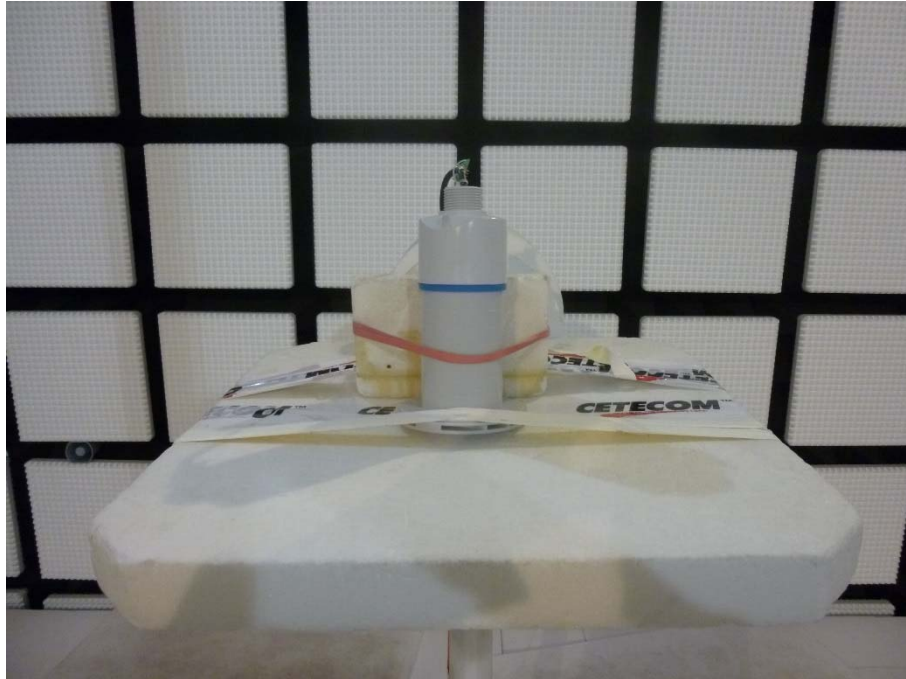
Photo 3: EUT at the anechoic chamber
