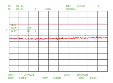
The offset (cable loss - amplifier gain + antenna factor) is calculated in the analyzer reading.
