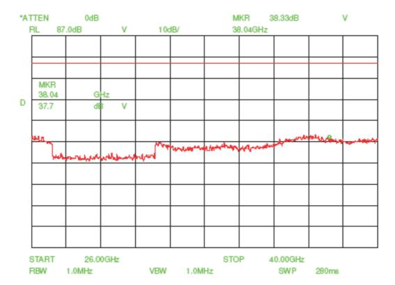
Calculation: Field strength = analyzer reading + cable loss - amplifier gain + antenna factor
