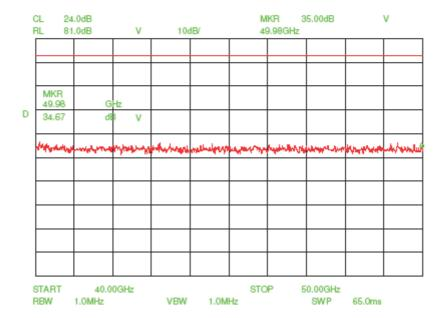
The offset (cable loss - amplifier gain + antenna factor) is calculated in the analyzer reading.
