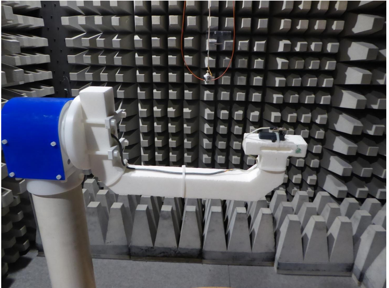
172289_E3_02.jpg: Test setup fully anechoic chamber
