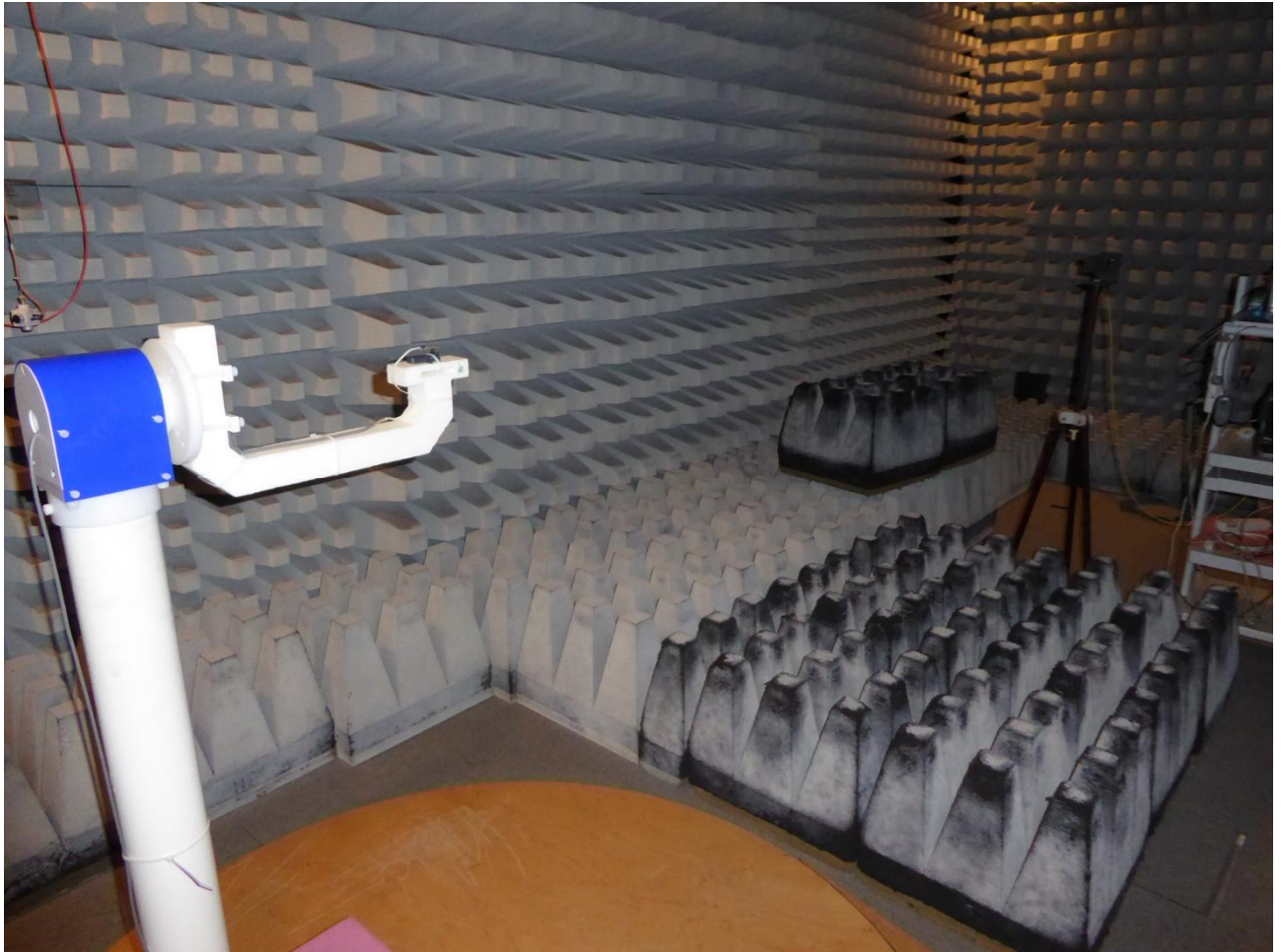
172289_E3_05.jpg: Test setup fully anechoic chamber
