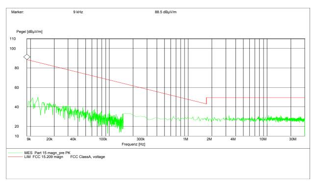
For peak measurement we use 100 kHz RBW/VBW For CISPR QP measurement we use 200 Hz from 9 kHz t 150kHz 9 kHz from 150 kHz to 30 MHz
