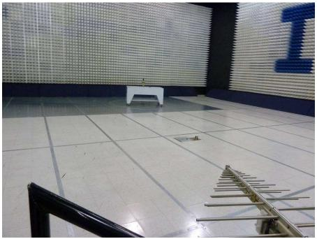
Radiated Emissions (Transmitter and Receiver spurious)
