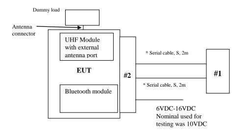
\* The DIG UHF-II Radio Module is a radio module intended to be installed in a host and does not contain any serial cables. The serial cables were used for setup purposes only which allowed control of the radio by test software. Radio tests were performed without these cables.
