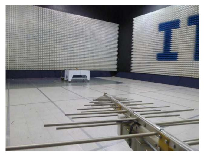
Electromagnetic Radiated Disturbance Setup Photograph
