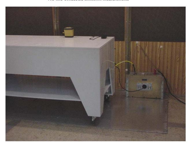
AC line-conducted Emission measurements
