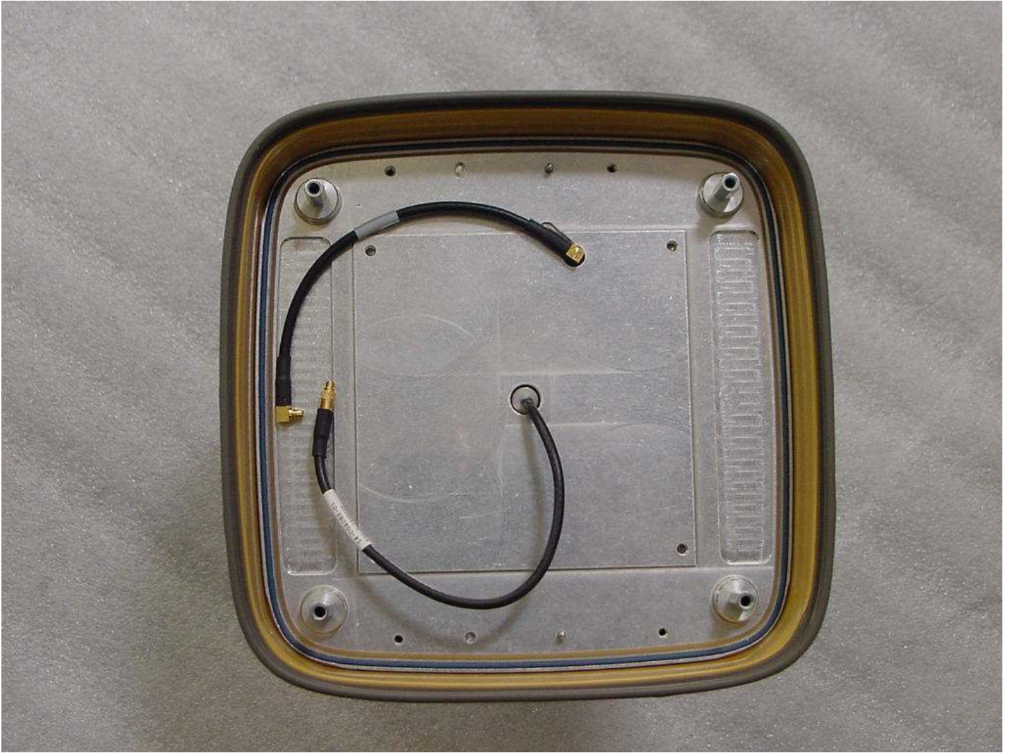
Interior of upper cover showing ground plane, modem connector cable (center) and GPS antenna connection
