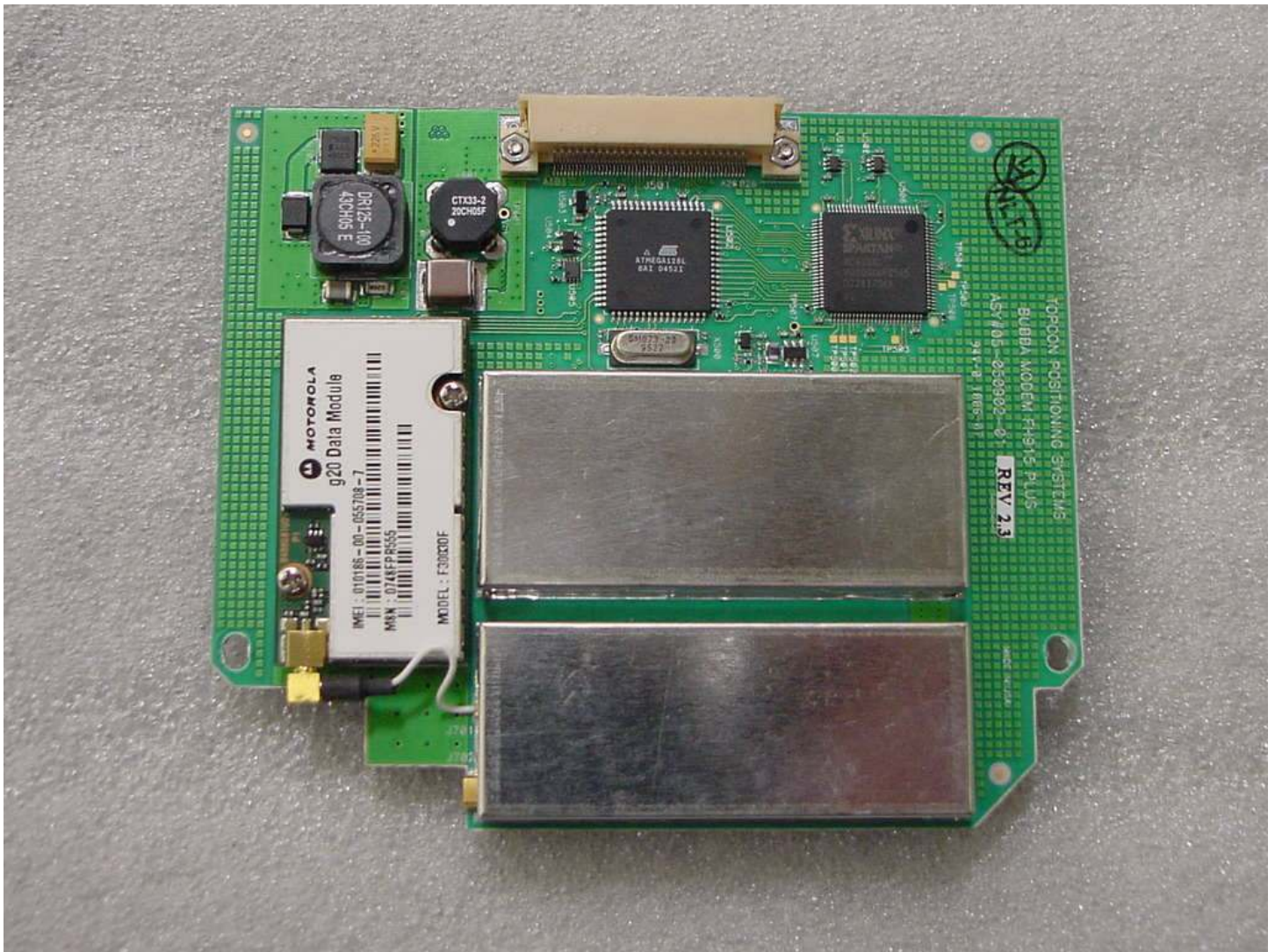
Bottom of FH 915+ modem board showing G20 module
