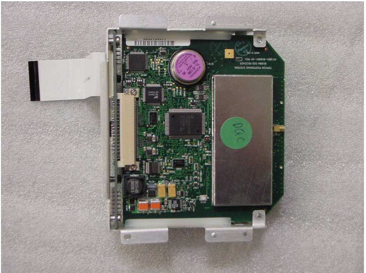
Card cage showing GPS board
