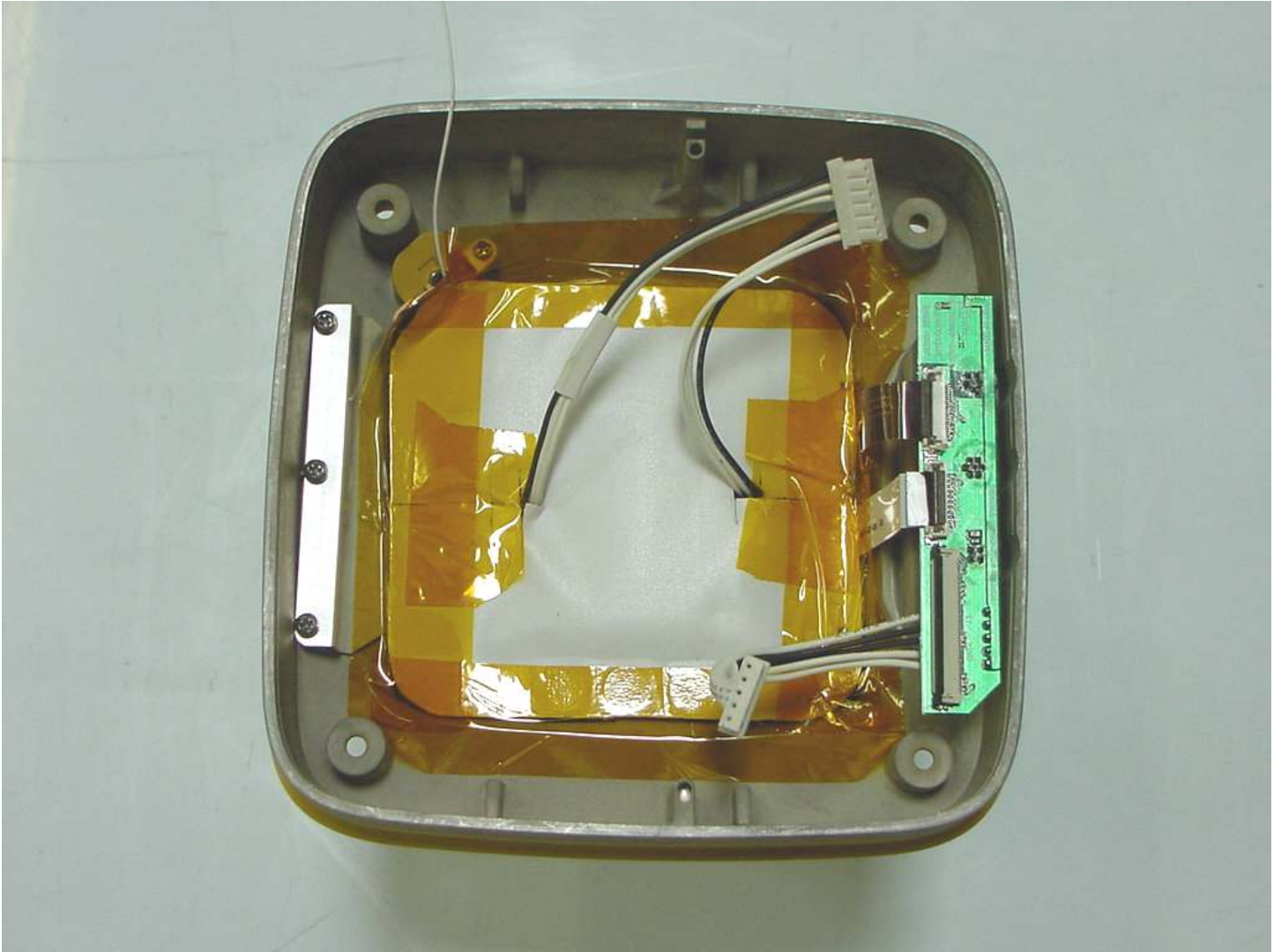
Bottom view of housing Interconnect on right side of photo
