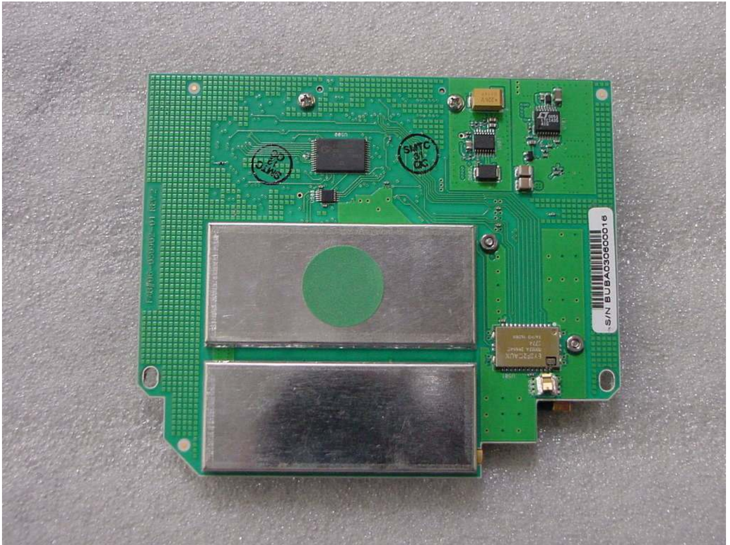
Top of FH 915+ modem board
