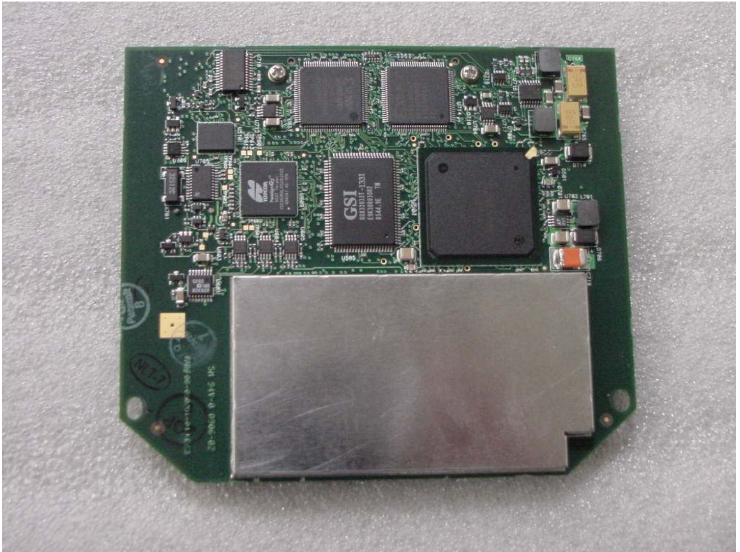
Bottom of GPS board
