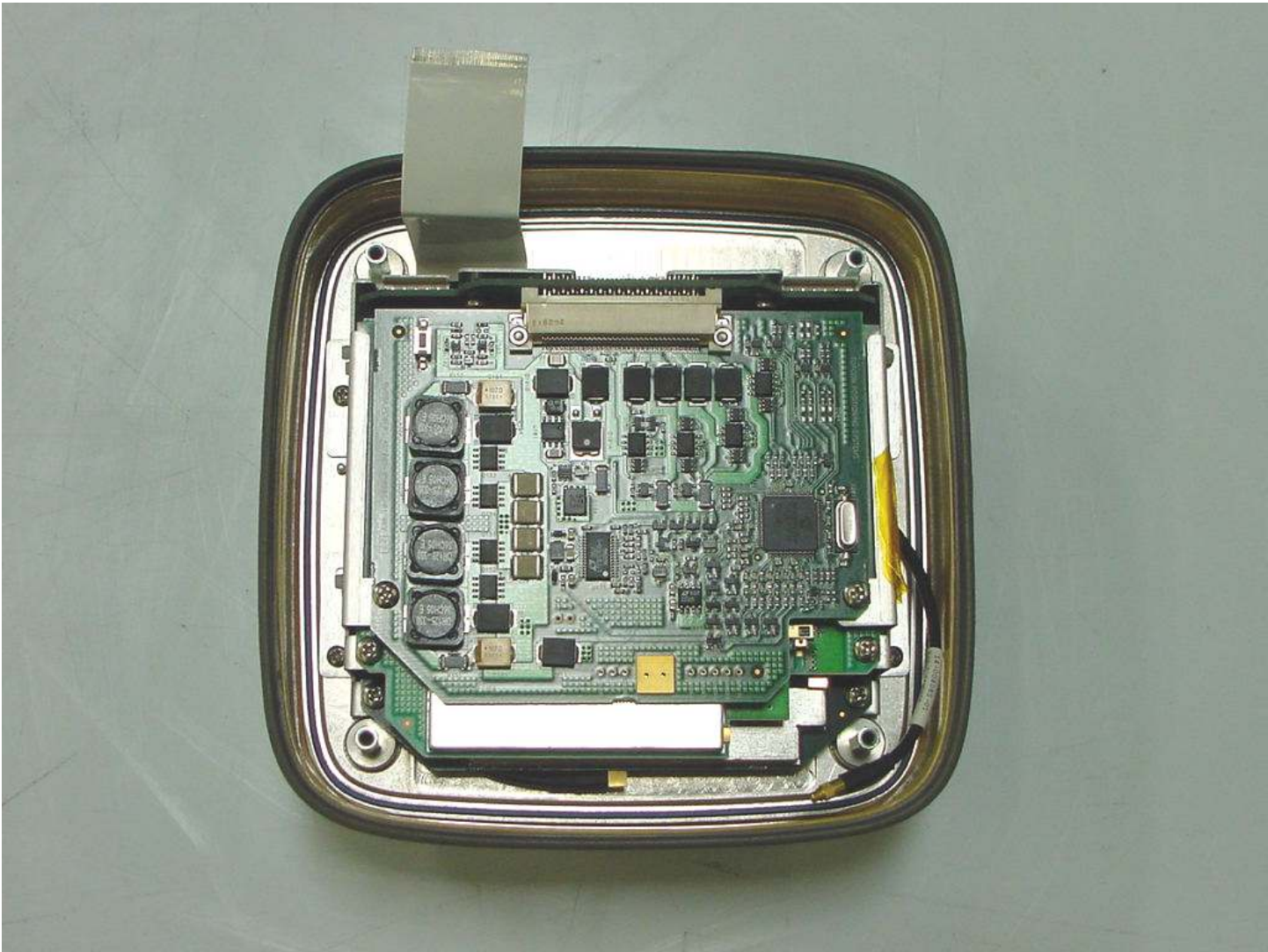
Bottom of card cage assembly showing powerboard
