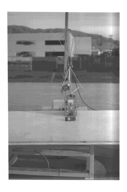
Test Setup Bi-Conical
