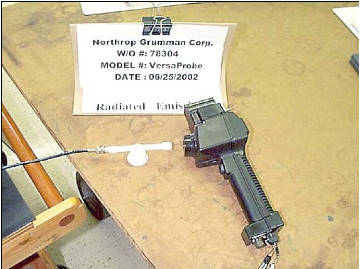
Radiated Emissions - Front View - H-Probe Antenna
