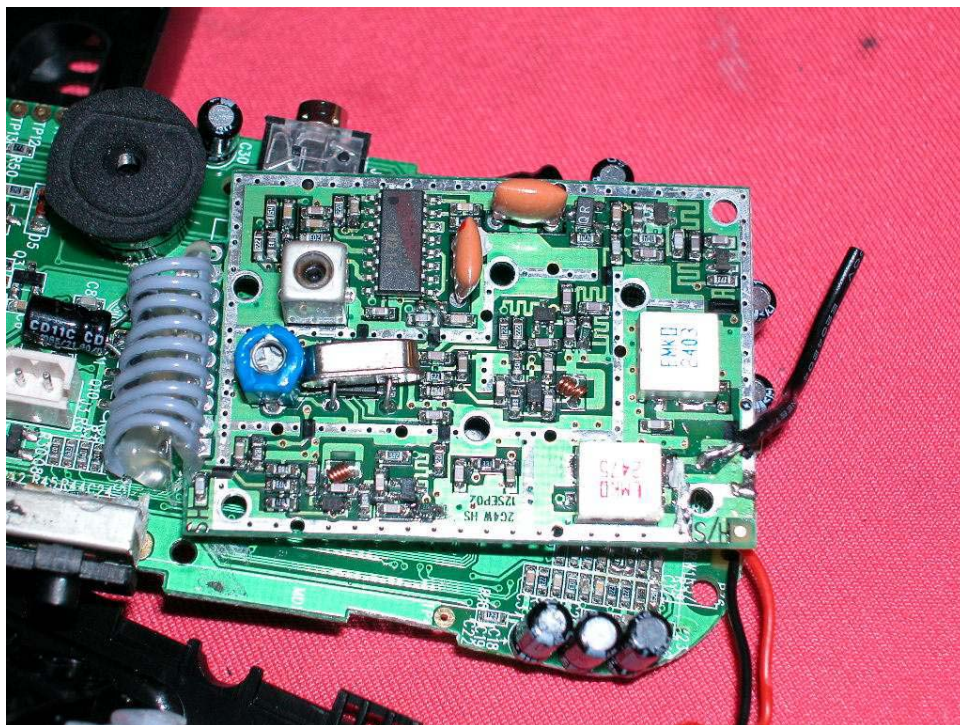
Handset Oscillator PCB comp side
