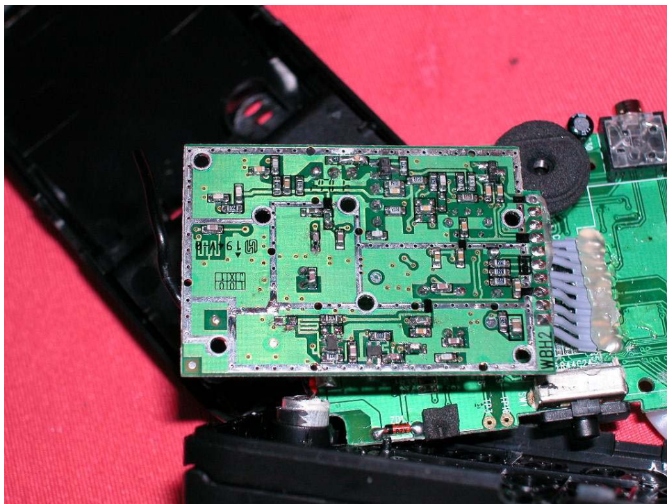
Handset Oscillator PCB solder side
