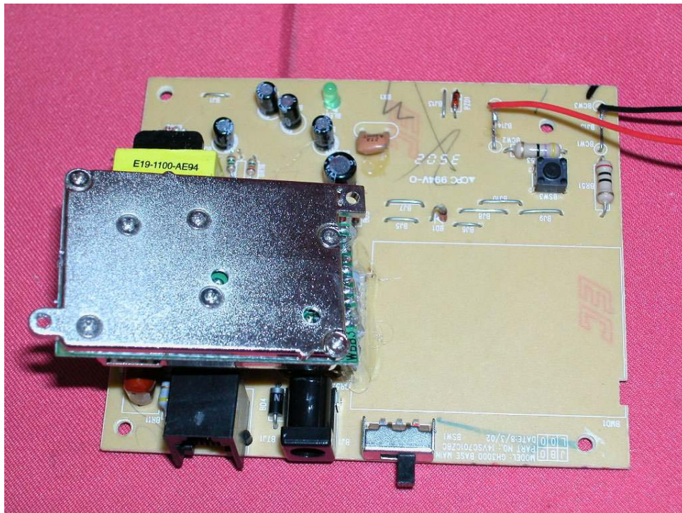
Base Main PCB comp side (view 2)
