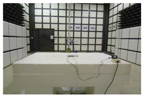
Radiated Emission Setup Photos (Above 1GHz)
