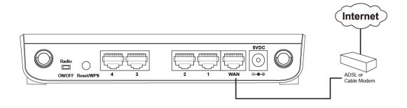
Connect your computers and network devices (network-enabled consumer devices other than computers, like game consoles, or a switch / hub) to an available LAN port of the router.
