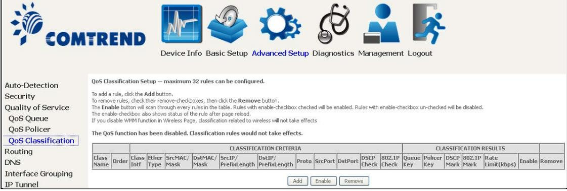
Click **Add** to configure a network traffic class rule and **Enable** to activate it. To delete an entry from the list, click **Remove**.
