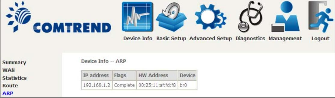
The screenshot shows the COMTREND web interface with a navigation bar containing icons for Device Info, Basic Setup, Advanced Setup, Diagnostics, Management, and Logout. On the left, a sidebar menu lists Summary, WAN, Statistics, Route, ARP (highlighted), and DHCP. The main content area displays 'Device Info -- ARP' with a table:
