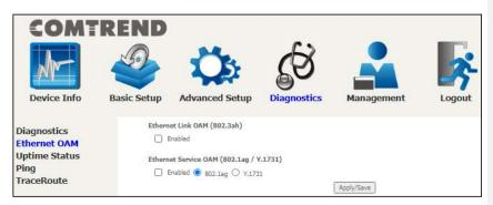
To enable Ethernet Link OAM (802.3 ah), click Enabled to display the full configuration list. At least one option must be enabled for 802.1ah.
