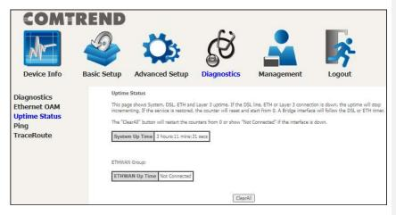
The "ClearAll" button will restart the counters from 0 or show "Not Connected" if the interface is down.
