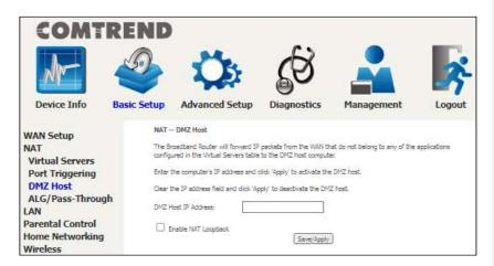
To **Activate** the DMZ host, enter the DMZ host IP address and click **Save/Apply**.
