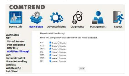
To allow/deny the corresponding ALG protocol, select Enable / Disable and then click the **Save** button. After reboot, the protocol will be added/removed to/from the system module.
