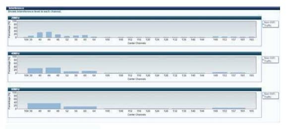
Shows the highest RSSI on each adjacent channel. Adjacent AP and associated stations are displayed for checking interference on those channels.
