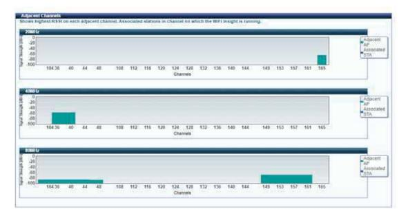
For each AP, the graph shows the control channel and extension channels. Extension channel is any channel spanned by the AP that is not a control channel.
