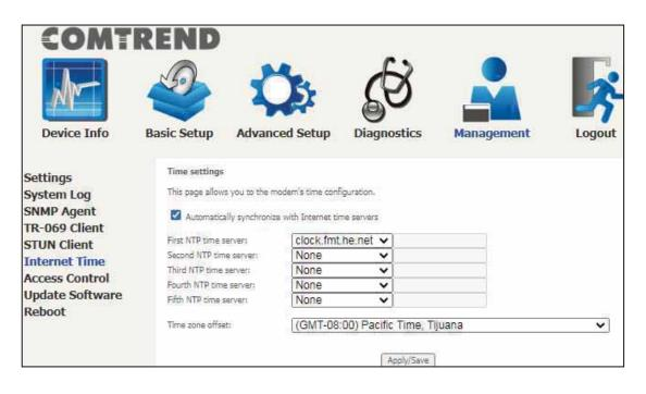
**NOTE:** Internet Time must be activated to use. See 5.4 Parental Control. The internet time feature will not operate when the router is in bridged mode, since the router would not be able to connect to the NTP timeserver.
