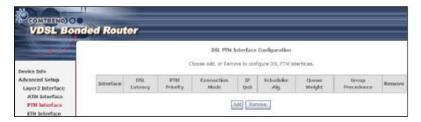
Click Add to create a new connection (see Appendix G - Connection Setup). To remove a connection, select its Remove column radio button and click Remove.
