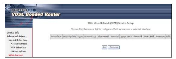
Click the Add button to create a new connection. For connections on ATM or ETH WAN interfaces see Appendix G - Connection Setup.
