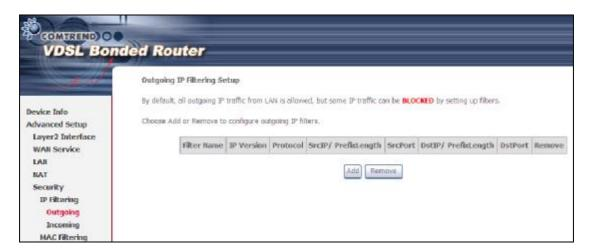
To add a filter (to block some outgoing IP traffic), click the Add button. On the following screen, enter your filter criteria and then click Apply/Save.
