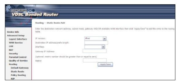
Select the IP Version from the drop down menu. Input the Destination IP Address, select the interface and input the Gateway IP Address. Then click Apply/Save to add an entry to the routing table.
