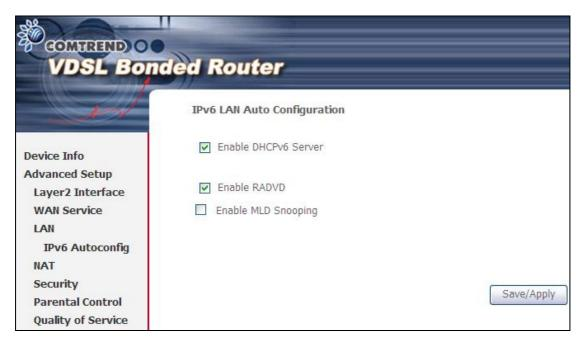
DHCPv6 Server: To enable DHCP for IPv6, select the Enable DHCPv6 server
