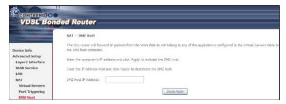
To Activate the DMZ host, enter the DMZ host IP address and click Save/Apply.
