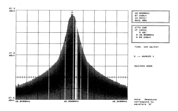
Result : The field strength of any emission within the operation band did not exceed 80 dB( $\mu$ V/m) for average value or 100 dB( $\mu$ V/m) for peak value. Refer to page 9 for the recorded value for the emission at the fundamental frequency.
