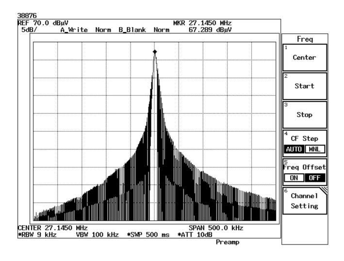
Result : The field strength of any emission within the operation band did not exceed 80 dB( $\mu$ V/m) for average value or 100 dB( $\mu$ V/m) for peak value. Refer to page 9 for the recorded value for the emission at the fundamental frequency.
