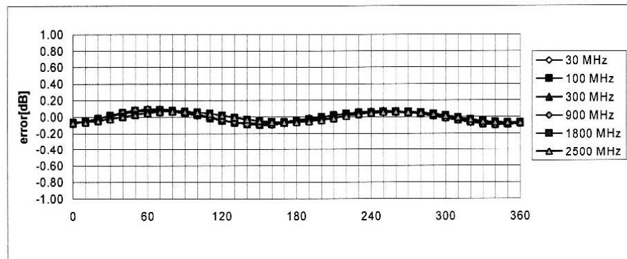
**Axial Isotropy Error  $< \pm 0.2$  dB**
