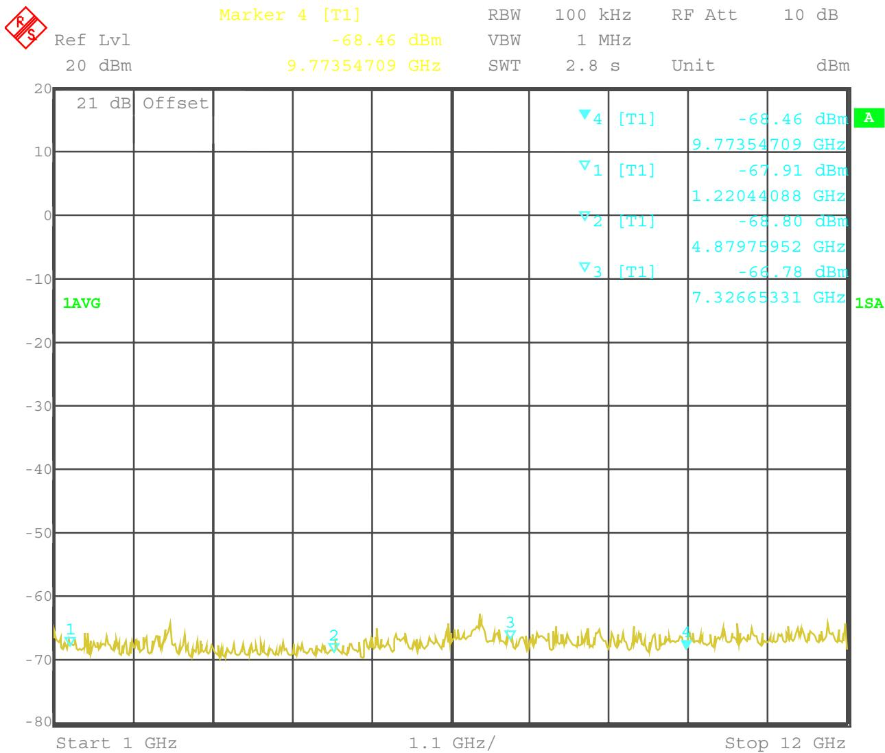
**This is only a scan. Final measurements were made below 1 GHz with 100 kHz RBW/VBW and a CISPR Quasi peak adapter , higher frequencies with 1 MHz RBW/VBW**
