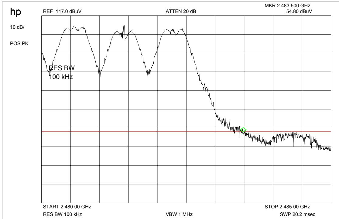
**Band-edge compliance of radiated emissions (4210/4215)****§15.247 (c)****This measurement was made to show, that the radiated emissions complies to the rules.**
