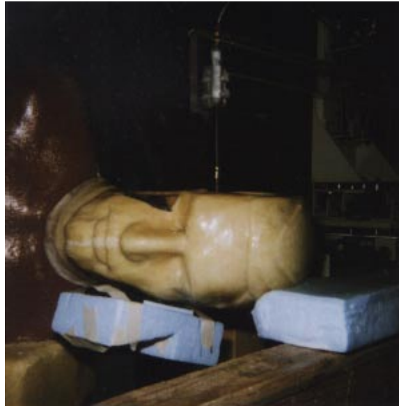
Fig. 2. The Siemens portable telephone (Model 4000 in this case) held against the phantom model of the head for measurement of SAR distribution.
