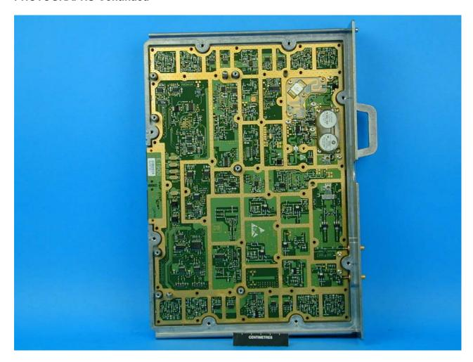
Photograph Number 14 - Internal -Base Band Board
