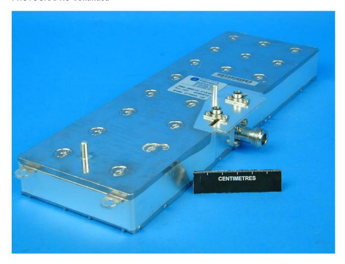
Photograph Number 7 – Internal – RF Filter
