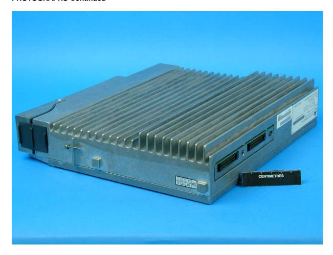
Photograph Number 20 – 24 DC PSU – Rear View
