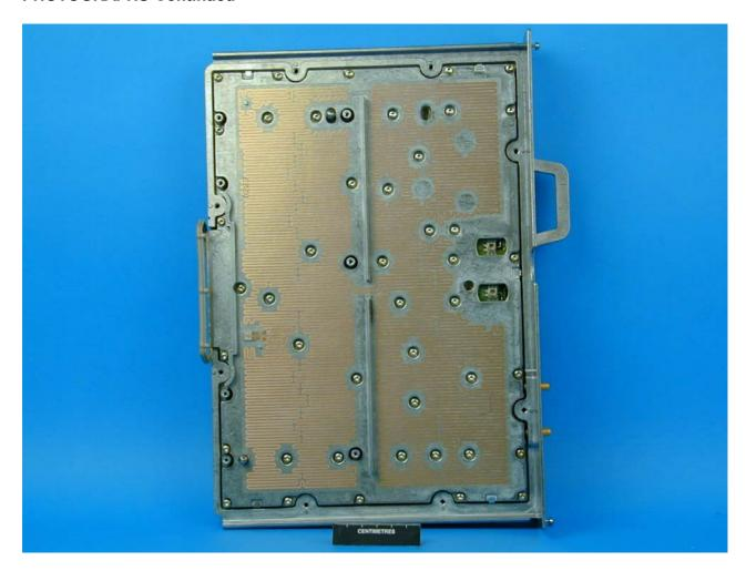
Photograph Number 9 – Internal –RF Filter and Small PCB Removed
