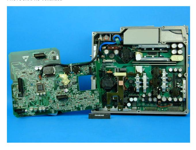
Photograph Number 24– 24 DC PSU– Internal – Top PCB Removed Shows Rear of Top PCB & Main PSU Circuitry
