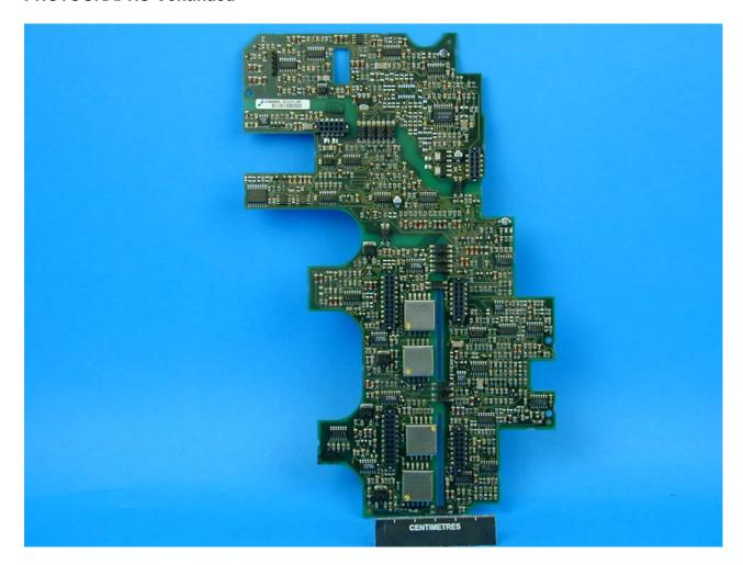
Photograph Number 32 – 110 AC PSU – Internal – Top PCB
