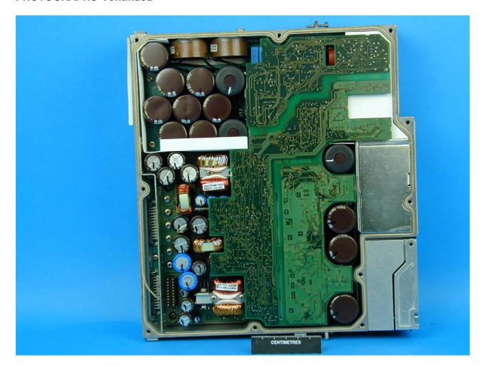
Photograph Number 31– 110 AC PSU – Internal – Top Cover Removed
