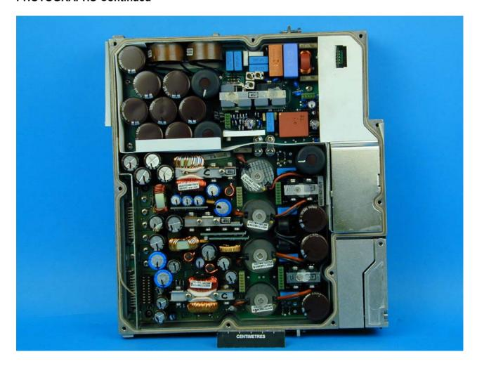
Photograph Number 35 – 110 AC PSU – Internal – Main PCB Circuitry
