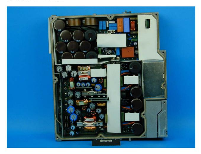
Photograph Number 34 – 110 AC PSU – Internal – Main PCB Circuitry
