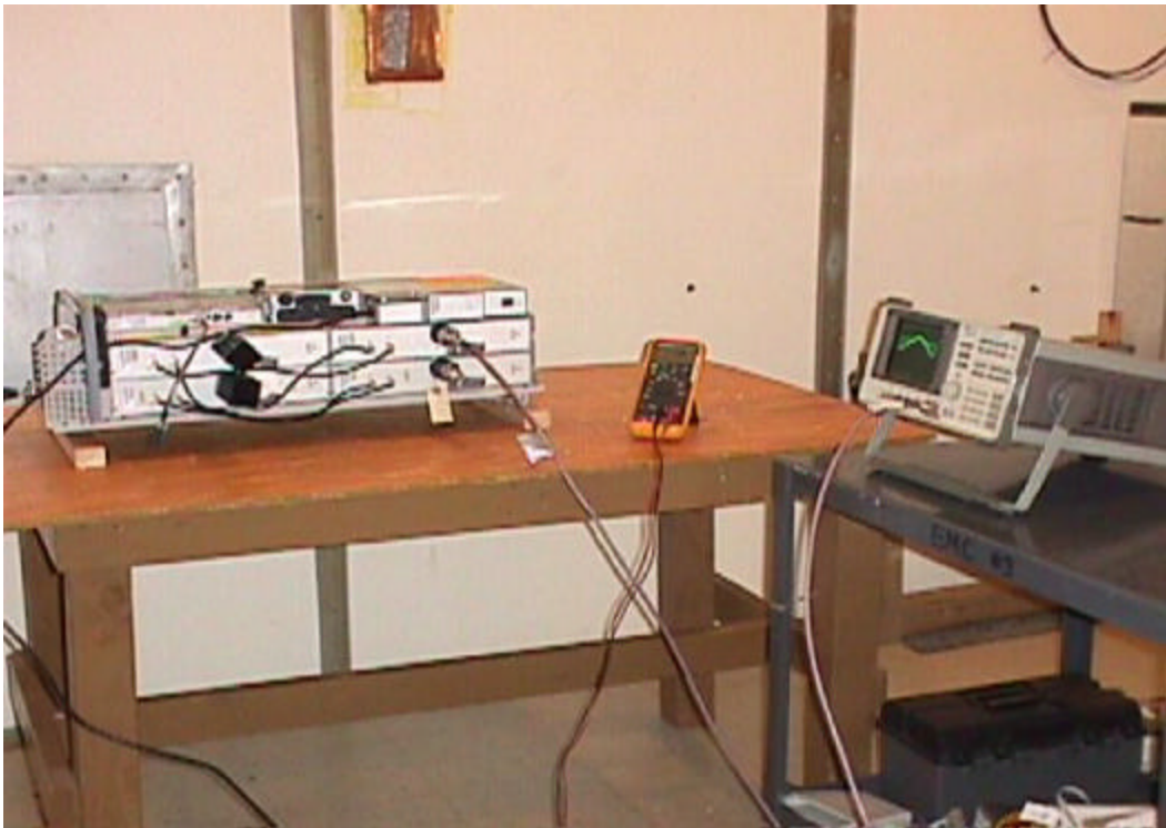
Photograph of Antenna Conducted Spurious Emissions Test Configuration
