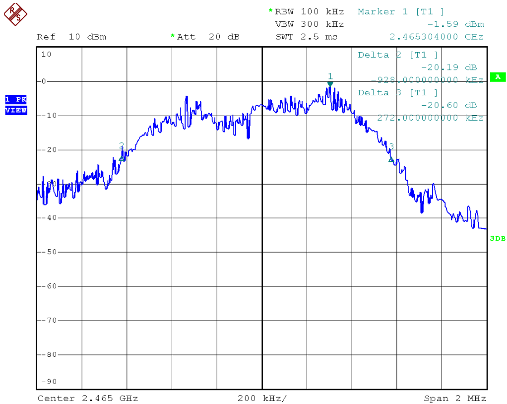
Figure 68 - 20dB Bandwidth measurement (fc=2465MHz) at FH4T mode
