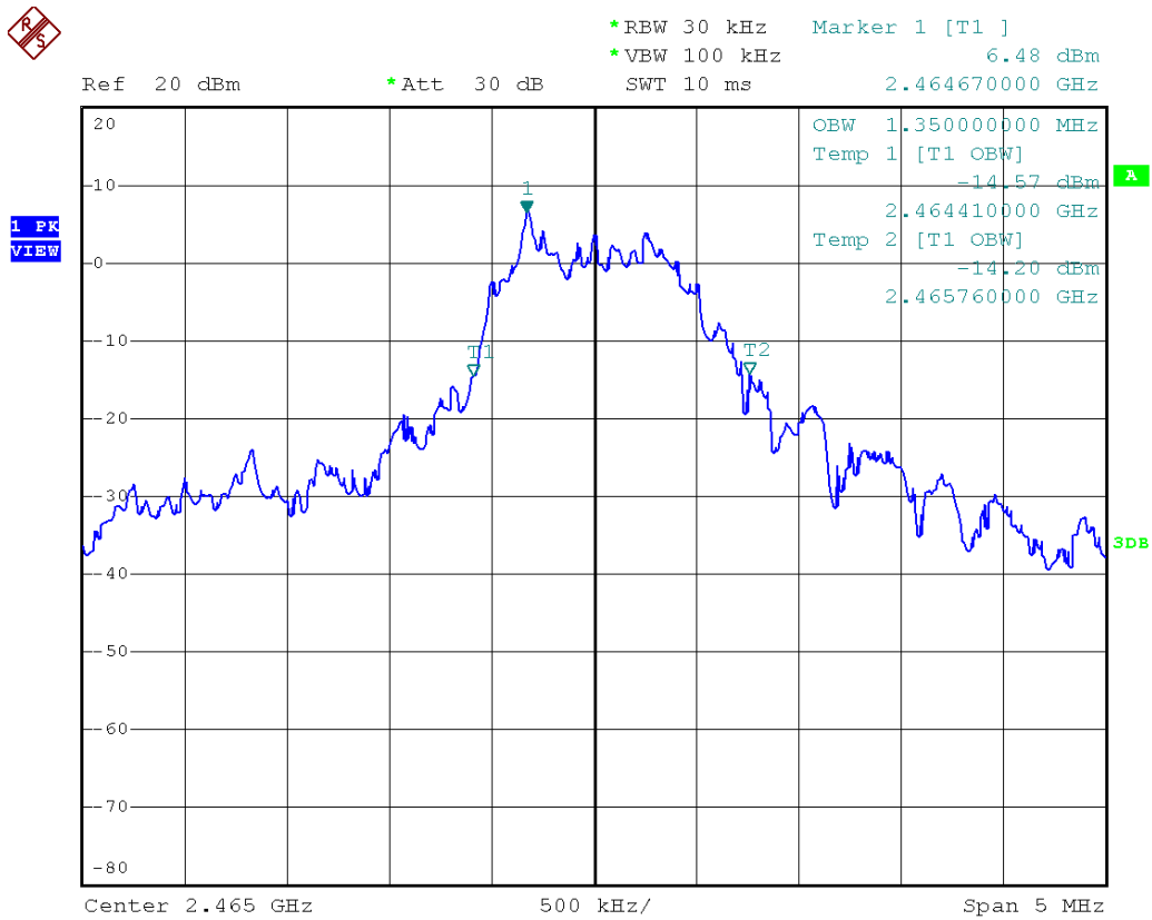
Figure 40- 99% Bandwidth Measurement (fc=2465MHz)
