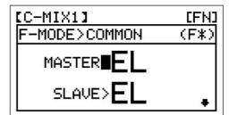
MASTER setting range is EL (Elevator), AI (Aileron), TH (Throttle), RU (Rudder), GY (Gyro), and PI (Pitch). The default setting is EL (Elevator).
