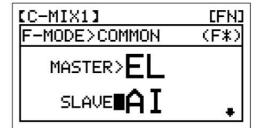
SLAVE setting range is EL (Elevator), AI (Aileron), TH (Throttle), RU (Rudder), GY (Gyro), and PI (Pitch). The default setting is EL (Elevator).
