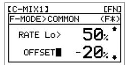
OFFSET setting range is -100% to 100%. The default setting is 0%. Increasing the Offset percentage value will shift the neutral position of the Slave servo in one direction and decreasing the Offset percentage value will shift the neutral position of the Slave servo in the opposite direction.
