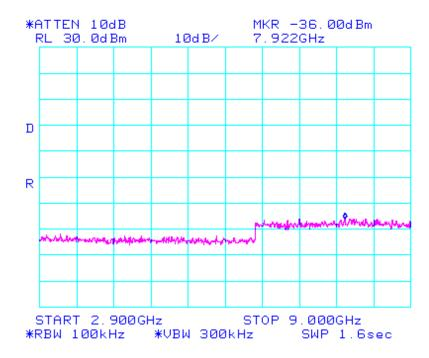
**6.6 TEST TYPE:** Intermodulation Spurious Emissions at Antenna Terminals
