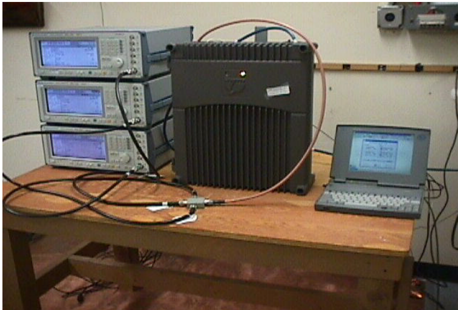
Photograph of Antenna Conducted Spurious Emissions and RF Power Output Test Configuration
