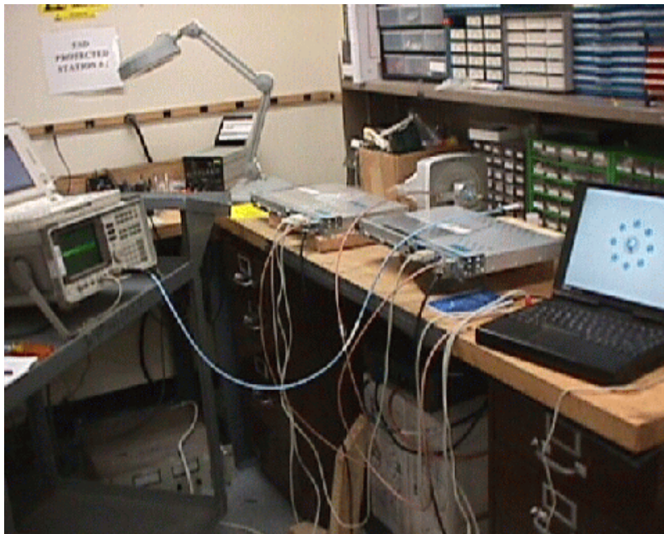
Photograph of Antenna Conducted Spurious Emissions and RF Power Output Test Configuration
