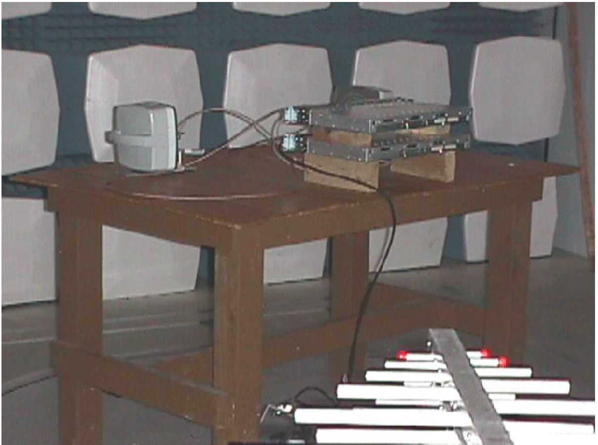
Photograph of Radiated Emissions Test Setup
