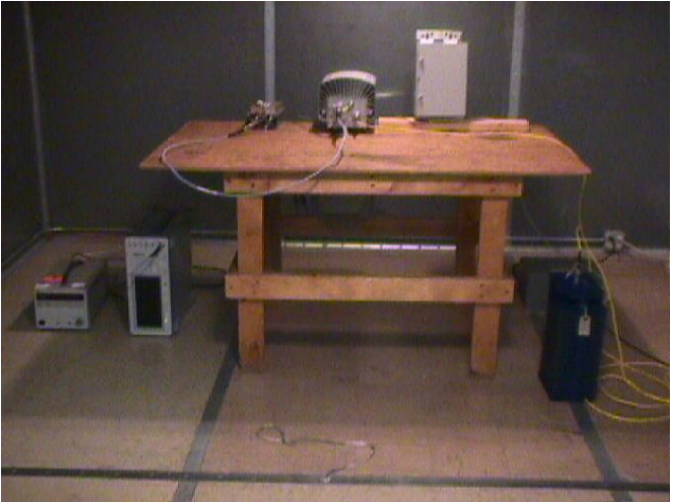
TEST SETUP OF LINE CONDUCTED EMISSIONS
