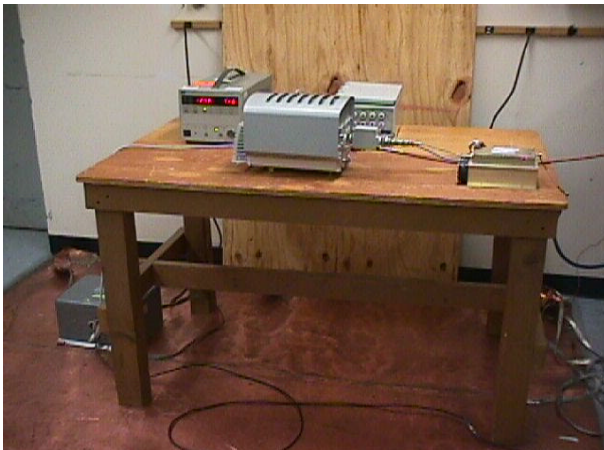
Photograph of Antenna Conducted Spurious Emissions and RF Power Output Test Configuration
