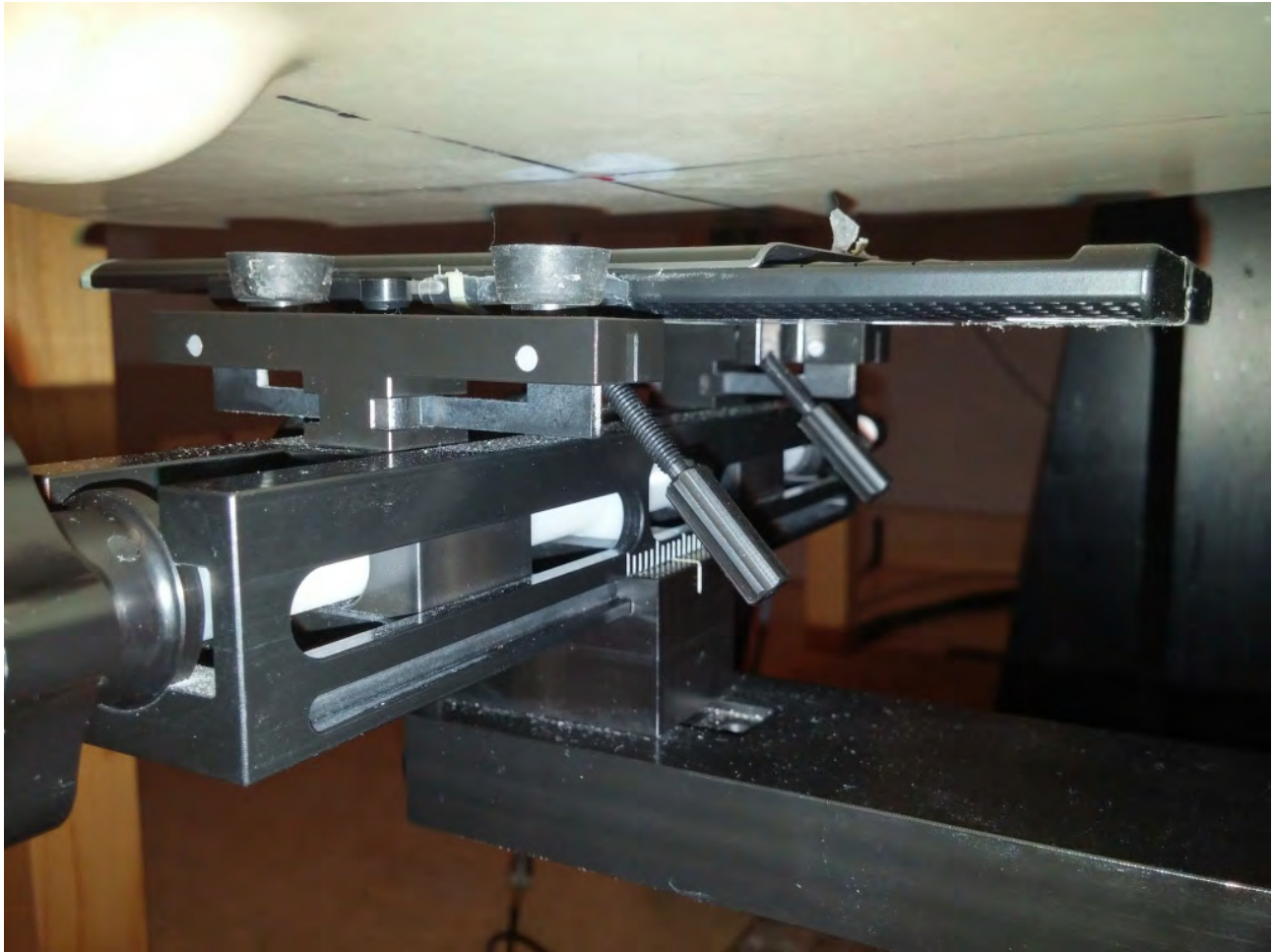
Figure E24. Body-worn configuration – Slider Closed (No Holster, front side 15mm away)
