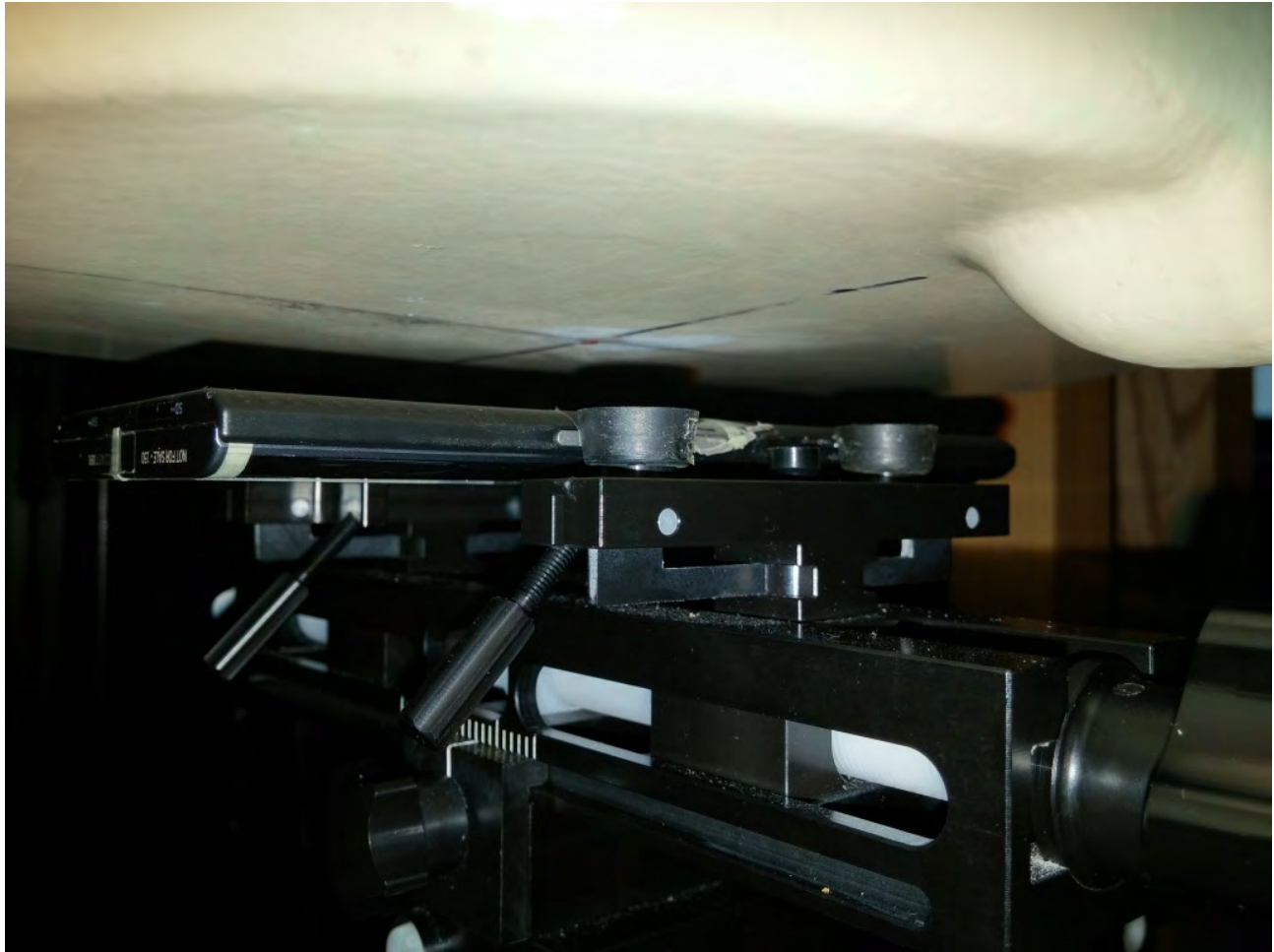
Figure E21. Body-worn configuration – Slider Closed (No Holster, back side 15mm away)
