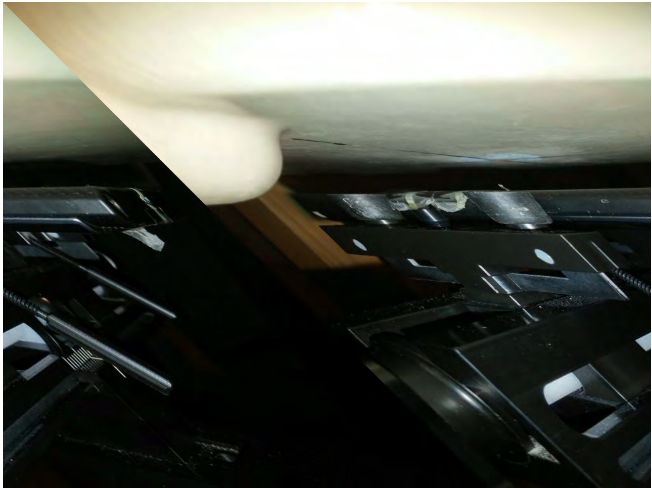
Figure E9. Hotspot configuration – Slider Closed (No Holster, back side 10mm away)
