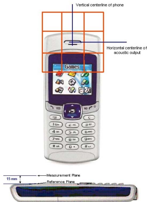
Figure 5.6-1: WD reference plane for RF emission measurement
