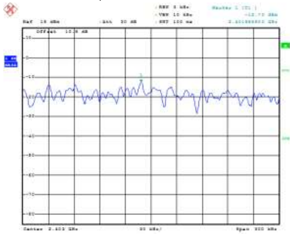
Figure 5-55: Peak Power Spectral Density LE, Channel 0
