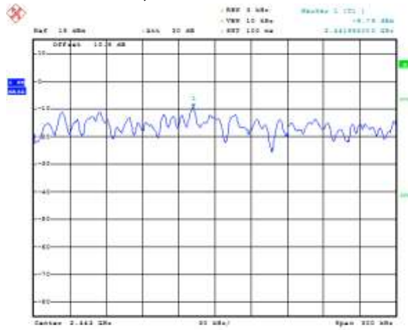
Figure 5-56: Peak Power Spectral Density LE, Channel 20
