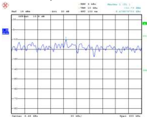
Figure 5-57: Peak Power Spectral Density LE, Channel 39
