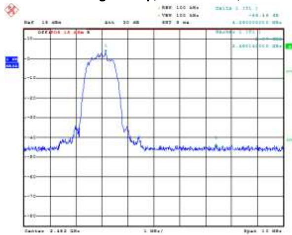
Figure 5-35: Band Edge Compliance Single Freq., Static PBRs, 3-DH5
