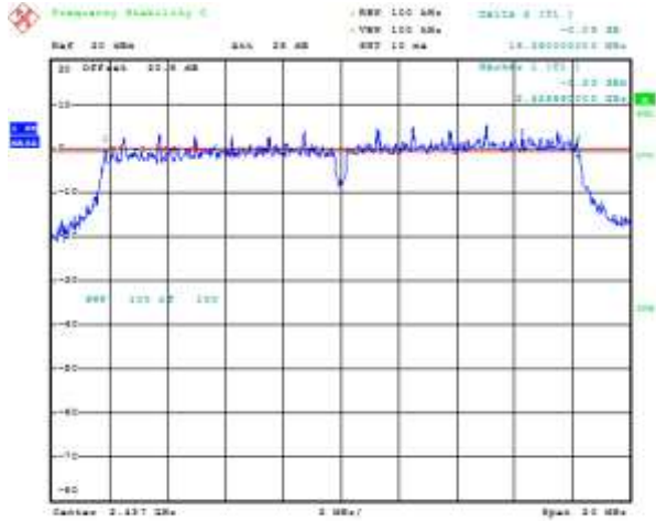
Figure 6-14: 6 dB Bandwidth Secondary, 802.11g, Channel 6, 6 Mbps
