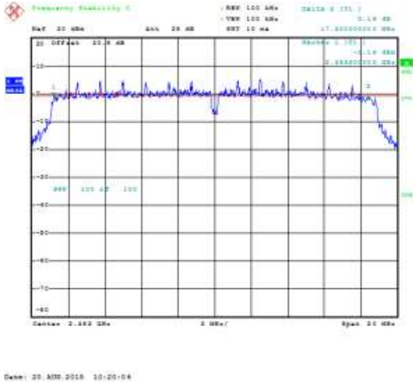
Figure 6-9: 6 dB Bandwidth Primary, 802.11n, Channel 11, MCS 0
