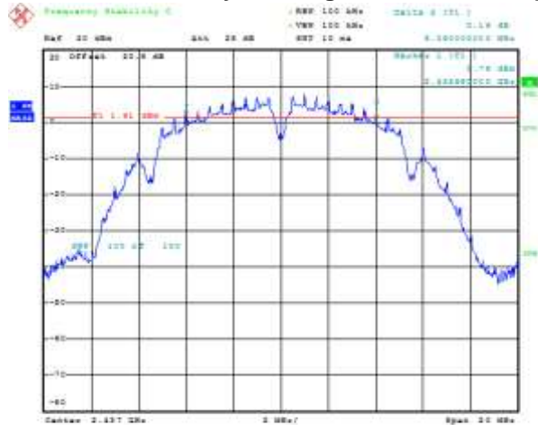
Figure 6-4: 6 dB Bandwidth Primary, 802.11g, Channel 1, 6 Mbps
