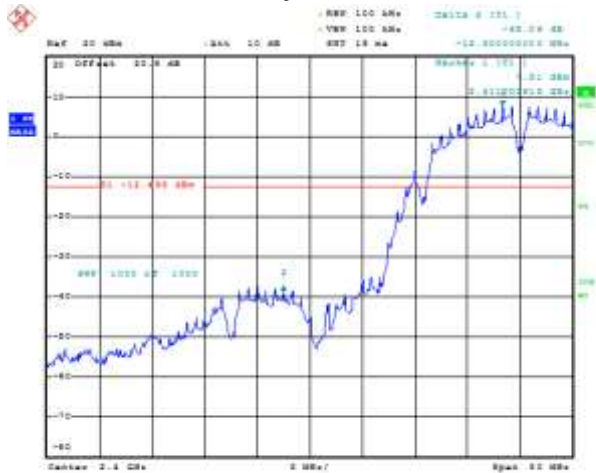
Figure 6-19: Band Edge Compliance Secondary, 802.11b, Channel 1, 1 Mbps
