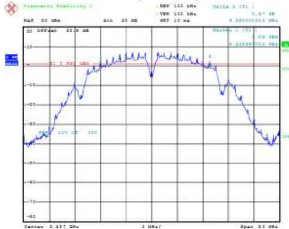
Figure 6-13: 6 dB Bandwidth Secondary, 802.11g, Channel 1, 6 Mbps
