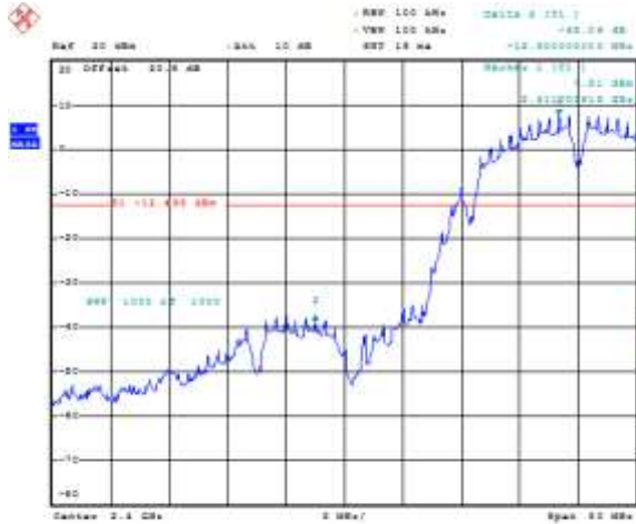
Figure 6-19: Band Edge Compliance Primary, 802.11b, Channel 1, 1 Mbps
