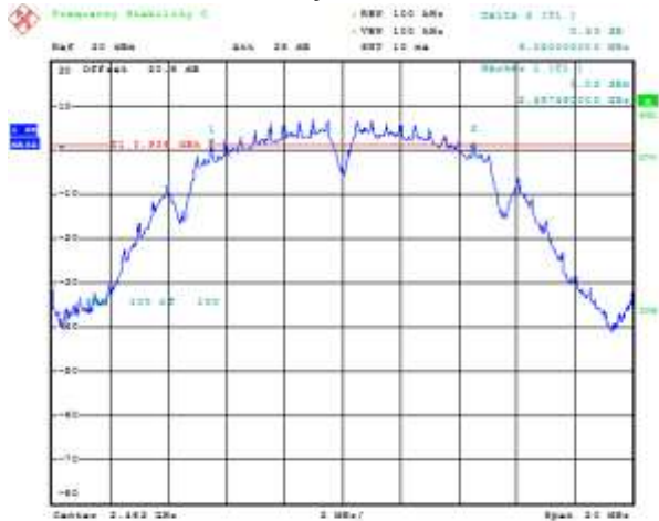
Figure 6-16: 6 dB Bandwidth Secondary, 802.11n, Channel 1, MCS 0
