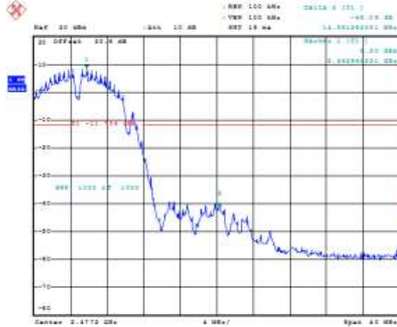
Figure 6-22: Band Edge Compliance Secondary, 802.11g, Channel 11, 6 Mbps
