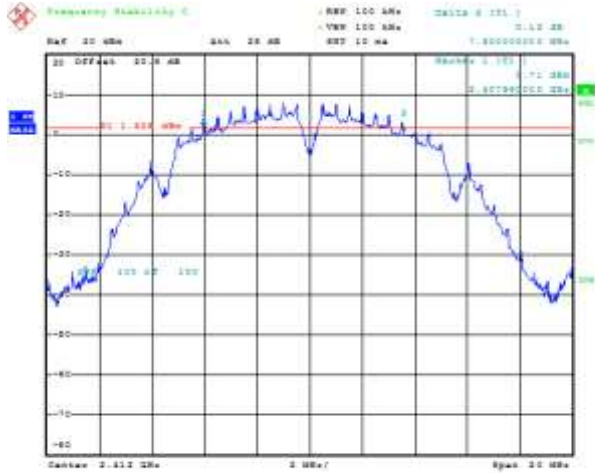
Figure 6-10: 6 dB Bandwidth Secondary, 802.11b, Channel 1, 1 Mbps
