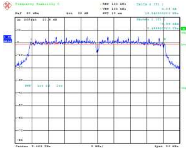
Figure 6-8: 6 dB Bandwidth Primary, 802.11n, Channel 6, MCS 0
