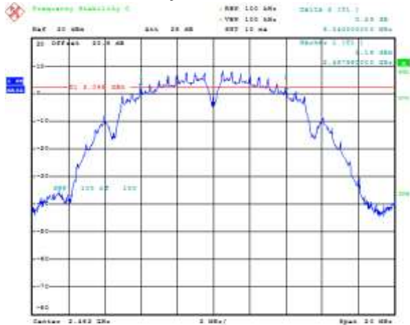
Figure 6-7: 6 dB Bandwidth Primary, 802.11n, Channel 1, MCS 0
